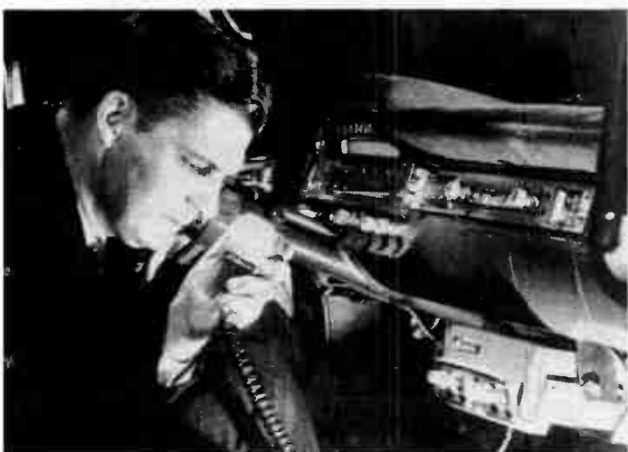
A new 100-watt transistorized two-way radio has been announced by Canadian General Electric Company Limited. It is the first transistorized two-way radio in the 100-watt category to be packaged in a case as small as four inches high, 8 1/2 inches wide, and 15 inches long.
