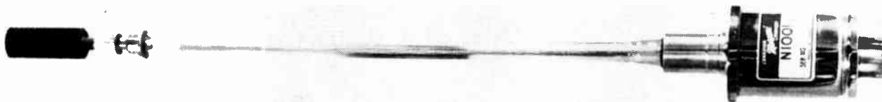
Figure 3 — Canadian Marconi Company Travelling Wave Tube — type N1001/B201. This tube delivers in excess of 100 watts in the 2000 Mc/s frequency range, and offer extreme reliability.
