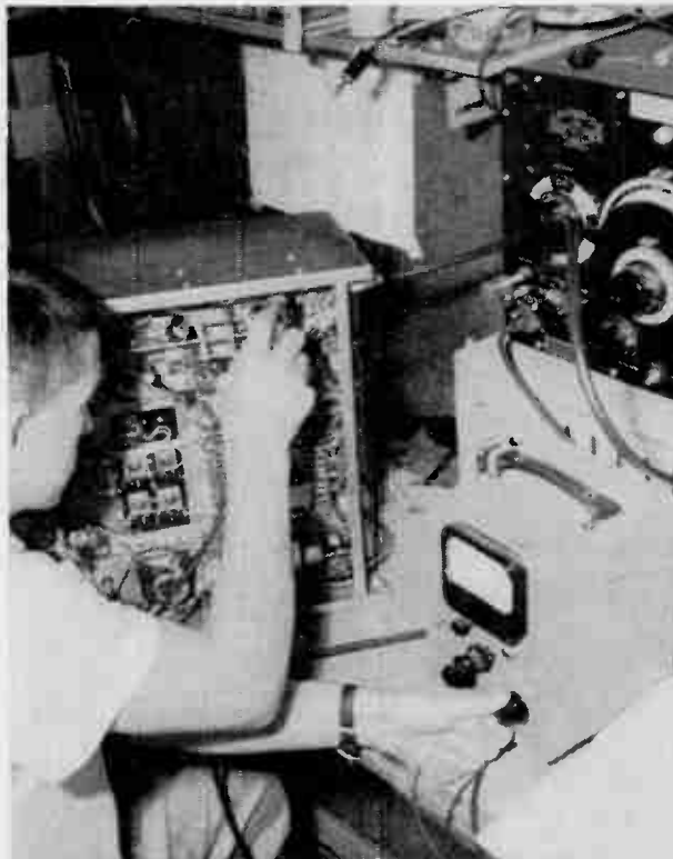
The bridging of an RSC Remote Control Unit, which is part of the AN/FRA-501 and AN/FRR-502 Remote Control Receiving System, is being carried out in the test and inspection department of T.M.C. (Canada) Ltd., Ottawa, manufacturers of communications equipment.
