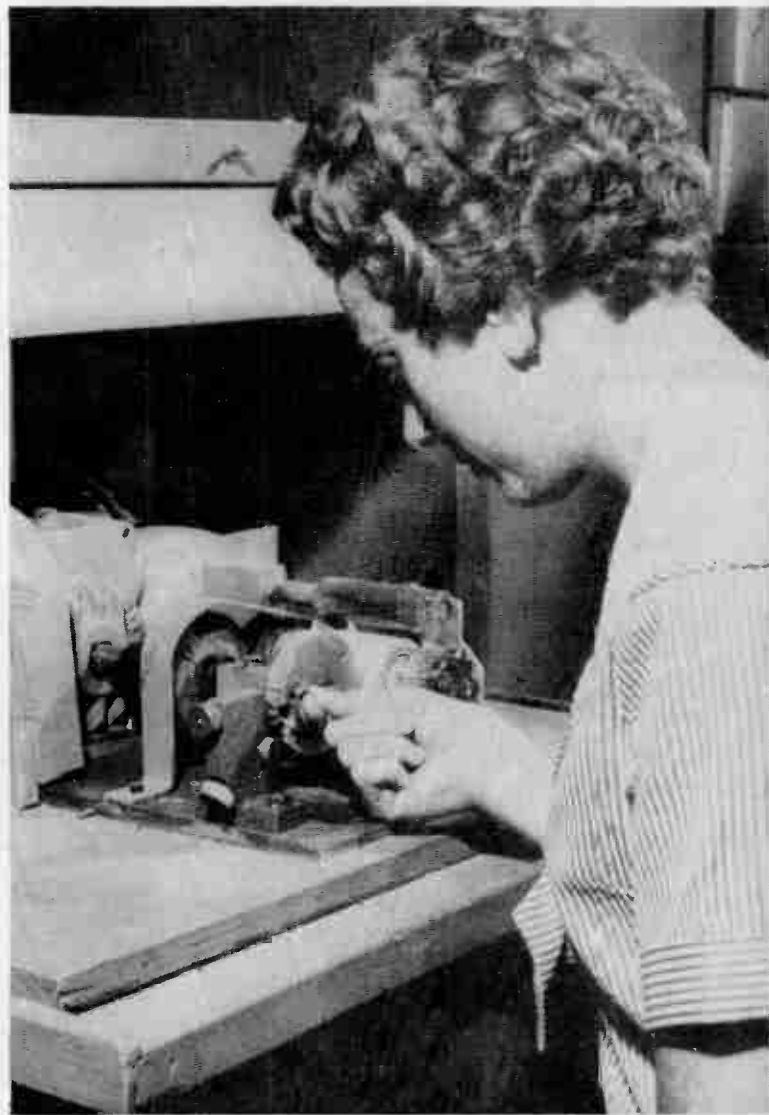
Among the hundreds of operations involved in the manufacturing of semiconductors at the Radio Valve Company Ltd. of Canadian General Electric in Toronto is the imprinting of the maker's name. Shown in the above photograph, an employee holds semiconductor at the printing machine which imprints the type and maker's name.
