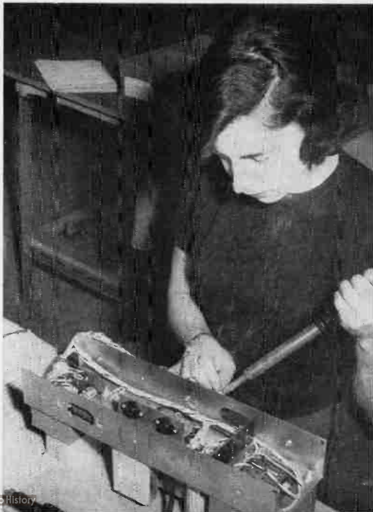
Below, technician at Pylon Electronic Development Company, Ltd., LaSalle, Quebec, is shown working on pre-wired sub-assemblies of power units, part of a growing line of proven solid-state devices manufactured by the company.
