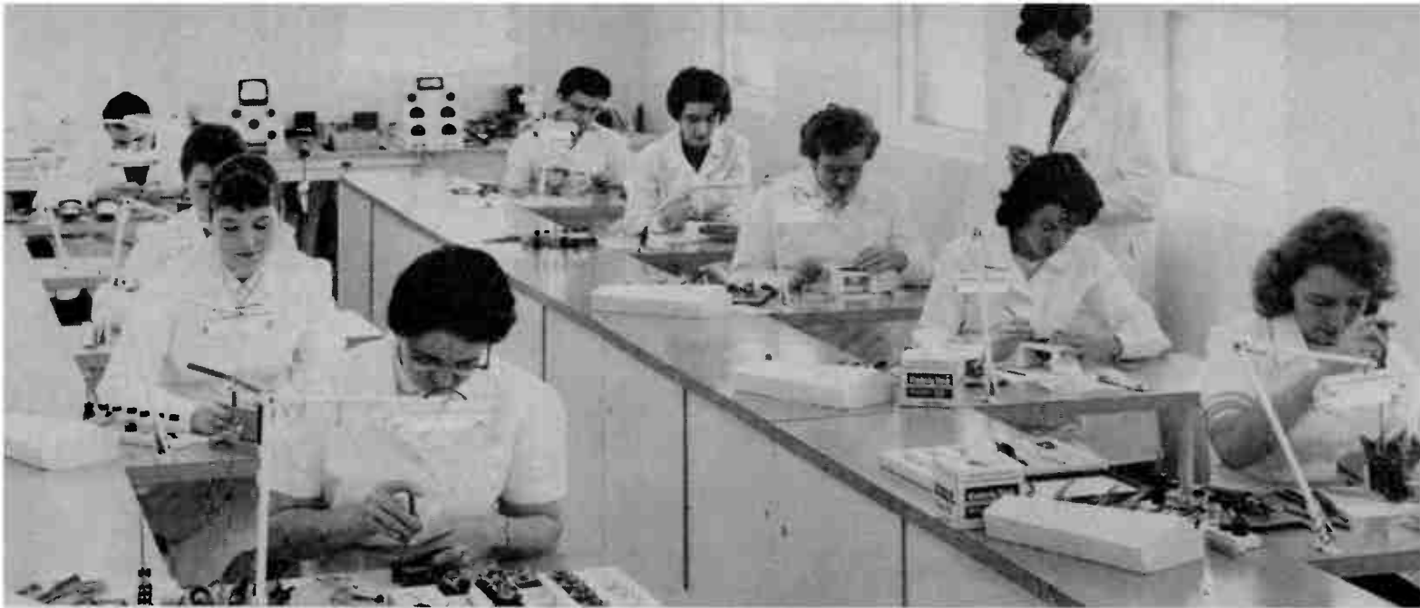
Canada's first "White Room" for meter making is now in full operation at Stark Electronic Instruments Limited, Ajax, Ontario. This "White Room" is especially designed for the manufacturing of meters with complete control of dust, humidity and temperature.
