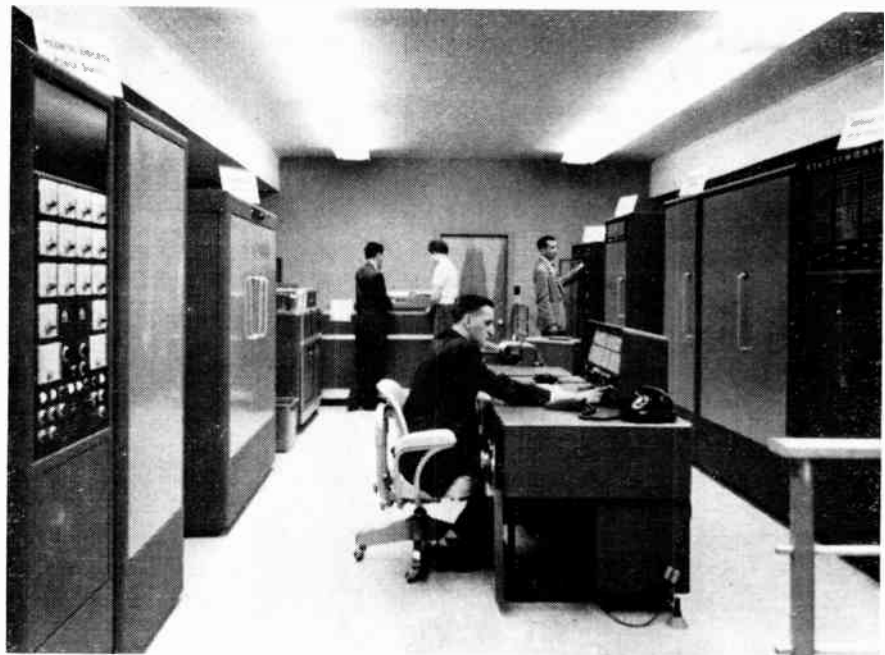
Interior view of Burroughs' new Electronic Data Processing Center in Ottawa shows the complete Burroughs 205 electronic computer system, one of the main units of the center which has been equipped to meet the data processing needs of Canadian government and business. The center also has a complete Burroughs E101 computer system. The center's facilities are available to serve Canada from coast-to-coast.
