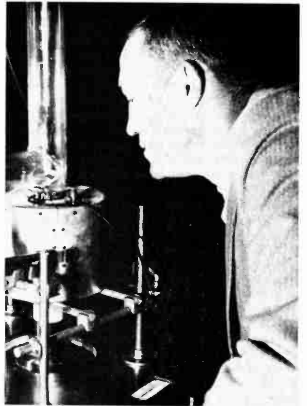
Small wonder that the pendant-shaped metal crystal suspended in the glass column commands the rapt attention of Salo E. Miller of Battelle Memorial Institute. The indium antimonide specimen, to be used in low-temperature transistors and infrared detectors, represents the purest crystal ever made of any compound. It has 99.99999+ purity.
