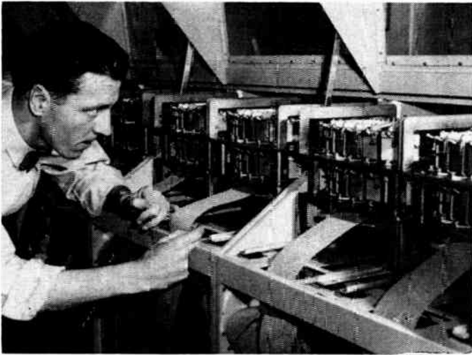
(Left) A Bell Telephone craftsman checks a roll of paper tape on a perforating machine on which are recorded details of long distance calls made via Direct Distance Dialing. These machines are only one of several complex units required for "DDD" service which was introduced at Toronto and Guelph during 1958 and is scheduled for Montreal in 1960.
