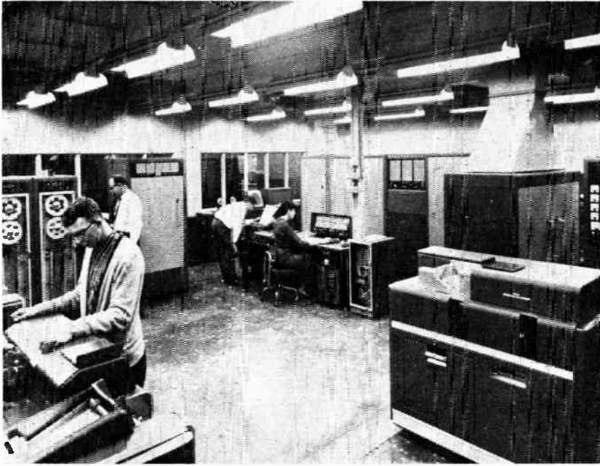
A view of the digital computer and personnel placed at strategic positions, namely the tabulator, the magnetic tape units, the flexowriter and the console.
