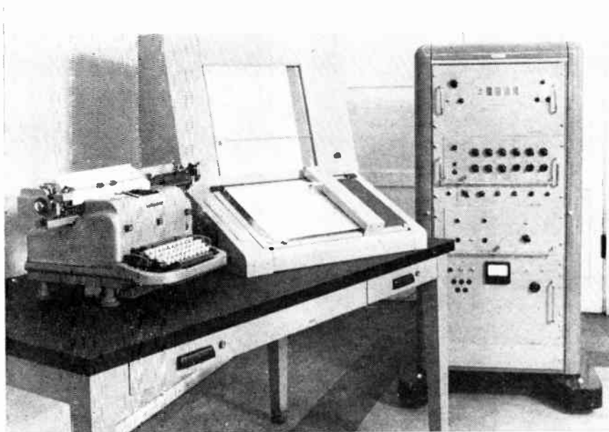
The K1028 Multi-Channel Trace Reader and associated equipment with separate linear and non-linear calibration facilities for each channel.
