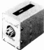
Transistor Servo Amplifier, Mod. AM-101 (AM-104 + AM-105). Application: High gain, 400 c. synchronous amplifier for highest accuracy velocity integrating servo-loop, using up to size 18 Bu. Ord. motor/tachometer generator. Built-in: power supplies, null voltage suppressor, tachometer generator phasing network, speed adjustment and quadrature rejection circuit.
