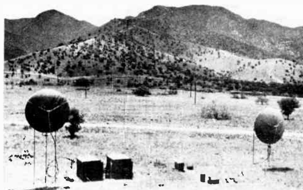
● Evaluating the air-transportable terminal for UHF transhorizon radio communication. The terminal includes two air-inflatable antennas, a receiver-exciter shelter (left) and a transmitter shelter.
