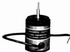
Magnetic Clutch, Model M-134. Body & Mounting: Similar to size 18 Bu. Ord. motor. All ball bearings. Max. speed 4000 r.p.m. Application: Servo mechanisms and computers. Energizing Power: 24 V.D.C., 3 watts. Min. Torque: 35 oz. inch.
