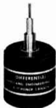
Differential, Model M-134. Body & Mounting: Similar to size 18 Bu. Ord. motor. All ball bearings. Application: Servo mechanisms and computers. Speed/Torque: symmetrical mechanical differential max. speed of any shaft 4000 r.p.m.; max. torque output 10 oz. inch.
