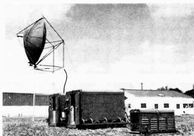
● Complete UHF transhorizon radio communication terminal, including two air-inflatable antennas, can be dismantled and shipped in the two enclosures that serve as shelters for receiving and transmitting equipment.
