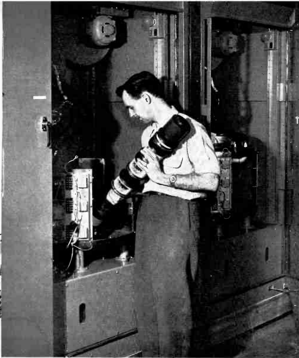
The Eimac high power amplifier klystron is installed in Collins Canada type 240E-2 one kw and 240D-1 10 kw troposcatter transmitters.
