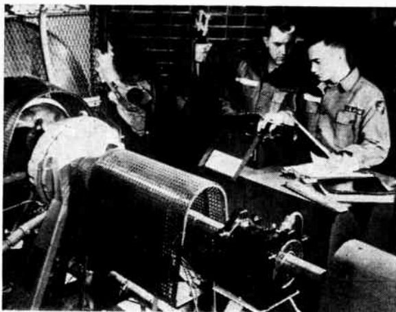
● Cadets discuss the results obtained with the SR-4 torque indicator. The black, cylindrical cartridge on the shaft in the foreground is the SR-4 torque pick-up.
