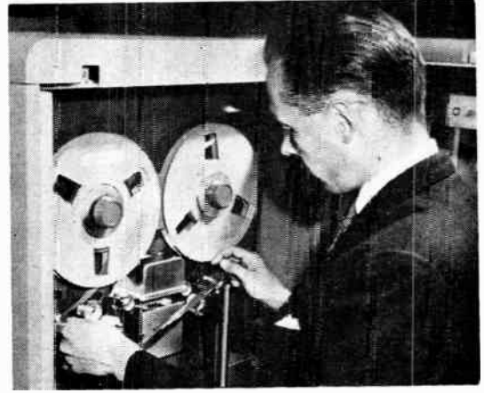
● One of the four Type 727 magnetic tape "read-write" units. These are auxiliary units of the new 650 electronic data processing machine installed by Du Pont of Canada.
