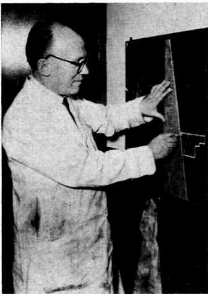
● The chief inspector, working out a technique for the ultrasonic testing of a particular casting. He is using a blackboard sketch of the casting and a 60° protractor to determine the angle of transmission of the Flaw Detector.
