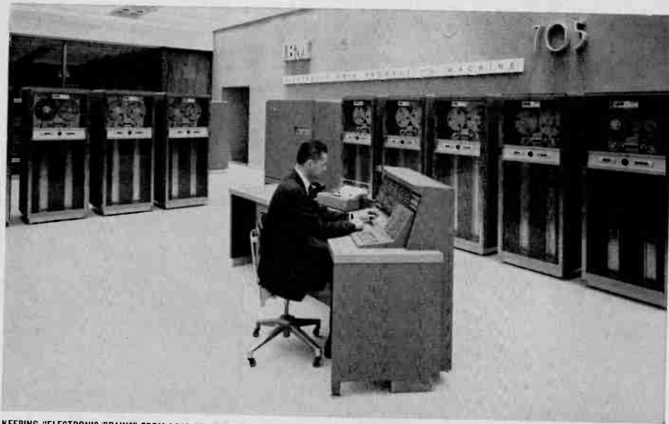
KEEPING "ELECTRONIC BRAINS" FROM LOSS OF MEMORY. One of science's greater marvels is IBM's 705 Electronic Data Processing Machine—which makes intricate calculations and logical decisions in millionths of a second. Heart of this electronic "wizard" is its main magnetic core memory. Designed for use with the machine's high-speed printer is the IBM 760 Control and
