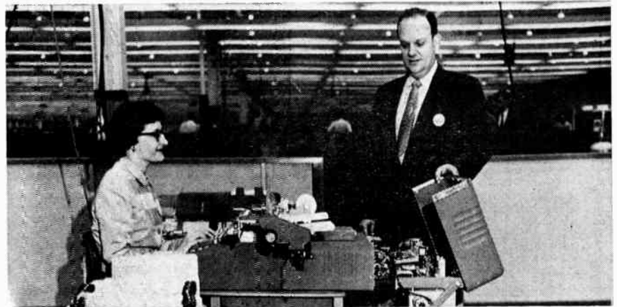
● T. C. Tudor, material control general supervisor at Convair-San Diego, holds cover open to show electromechanical intercoupler linking posting machine to punch card machine.
