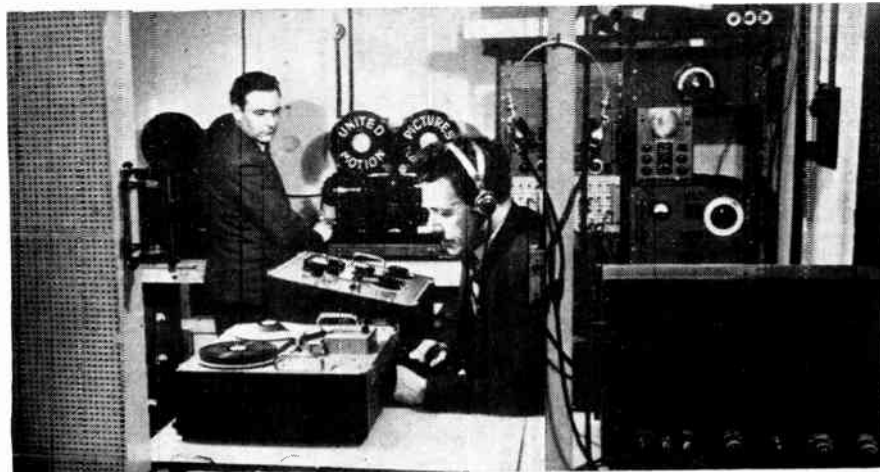
● A synchronous magnetic recorder recently installed is here seen transferring a recording to optical film.
