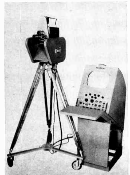
● Complete remote control operation of closed-circuit television cameras is provided by this unique "servo pan and tilt" system shown at right.
