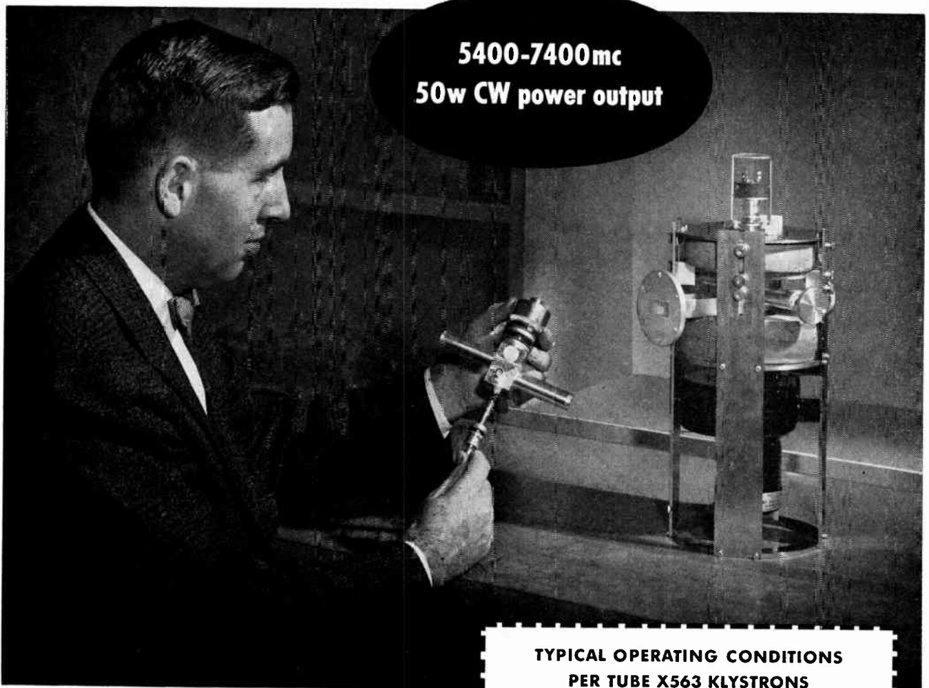
Eimac X563E, 5900-6400mc, and amplifier circuit assembly.
