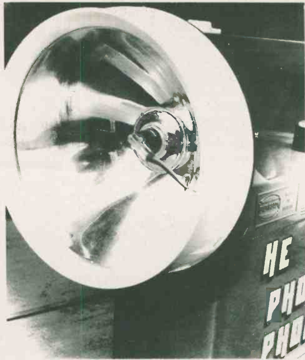
A view of the reflector modifications. The transistor should be placed with the small metal dot (just visible inside the protective gel of its case) towards the rear of the communicator. Some experimentation may be necessary to find the reflector's focal point exactly.
