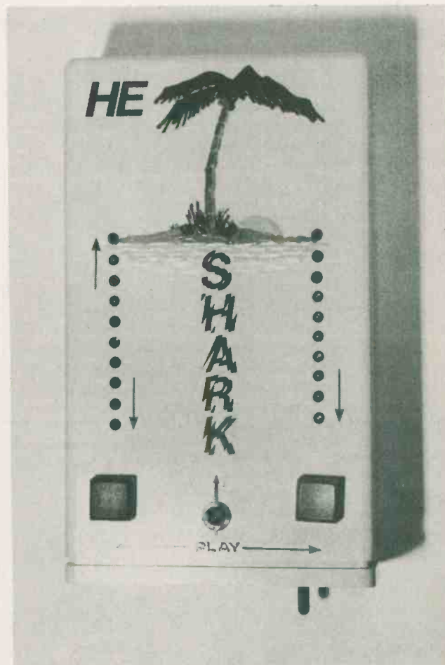
The case for Shark was made from a Vero box, the artwork on the case makes it look very attractive.
