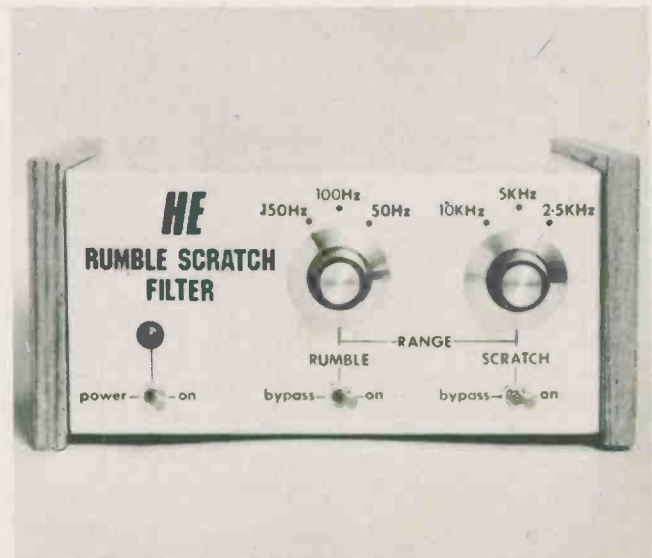
The finished filter. Note the two range switches, for the rumble and scratch sections, and the frequencies which they select.
