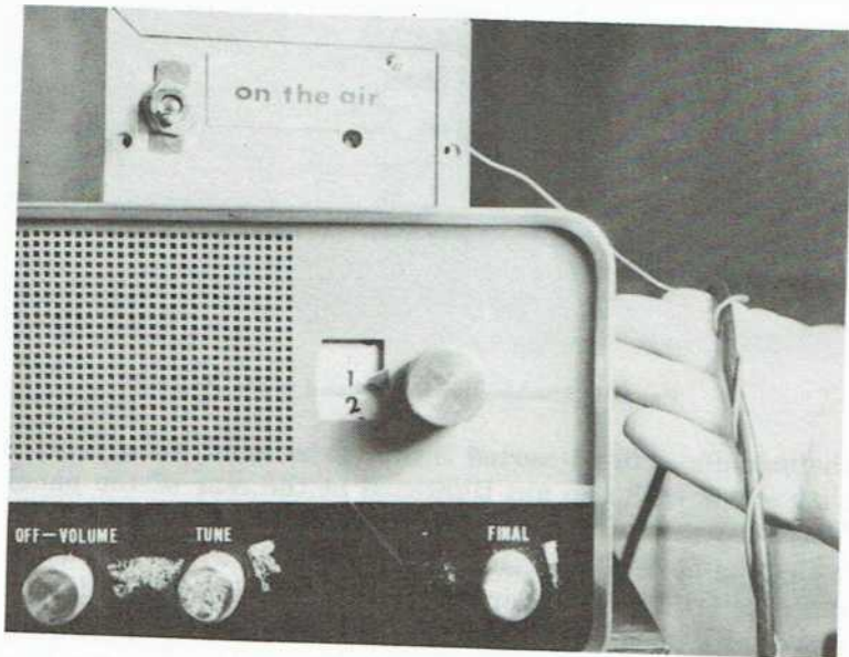
Fig. 17-10. Loop antenna around coaxial cable.
