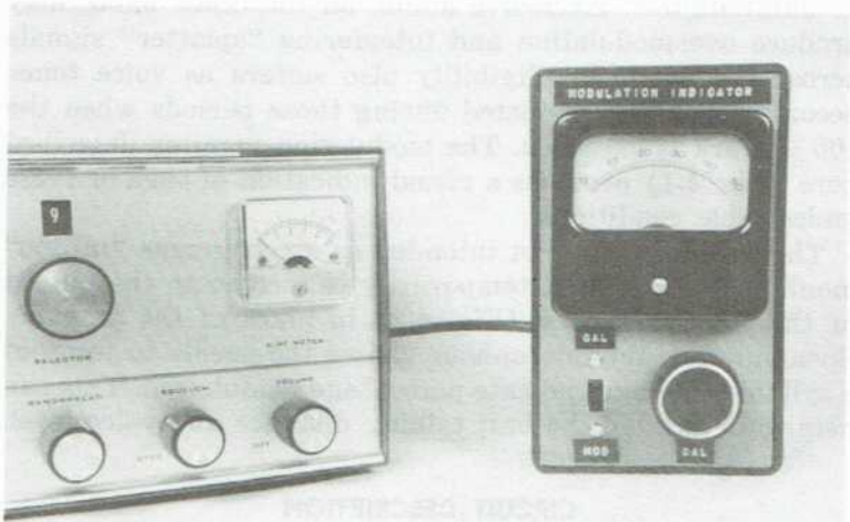
Fig. 4-2. Modulation monitor connected to output of CB transceiver.
