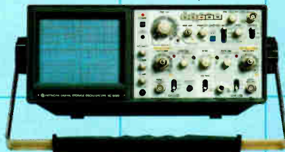
Hitachi VC-6020 • 20 MHz real-time • 1 MS/s digitizer • compact size • GPIB • Plotter output
