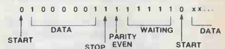
Fig. 3. Representation of the letter 'A' in seven-bit even parity code. Note that a '1' is a low voltage and a '0' is a high. The line normally sits at low or '1'.
