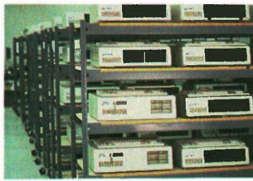
BEST computers undergoing their rigorous 48-hour automatic testing prior to shipping.
