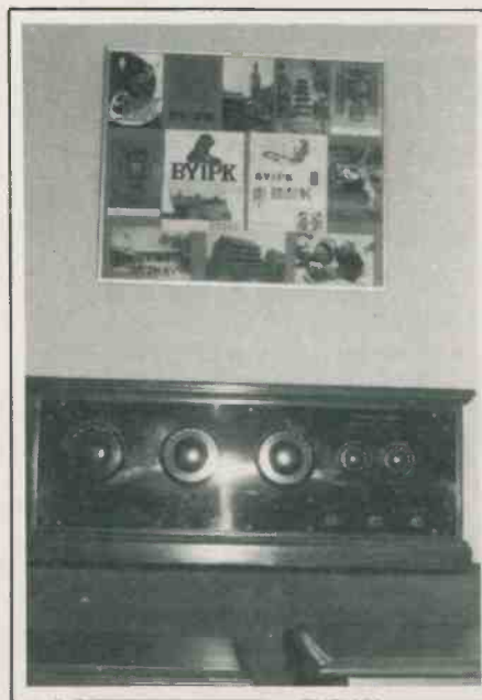
Some of Fred Hammond's DX cards confirming long-distance reception. Below is a Stromberg-Carlson receiver of the 1920's; the three RF stages had to be tuned exactly with each other. All photos by Dave and J.W. Essex.
