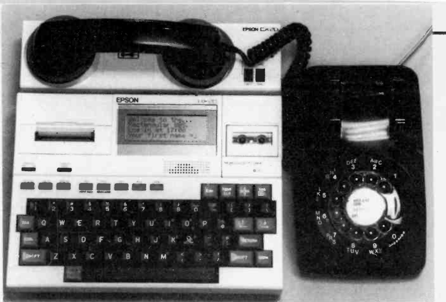
Portable computers such as the Epson HX20 shown above are a natural for journalists on assignment; textfiles can be sent to the publisher over telephone lines using either a direct-connect or a handset modem.
