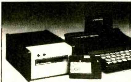
PICTURED IS TS1000, STRINGY FLOPPY DRIVE & INTERFACE 16K RAM AND A MICRO WAFER
