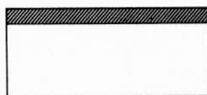
(a) OXIDATION: GROWTH OF SILICON DIOXIDE LAYER ON SILICON SLICE
