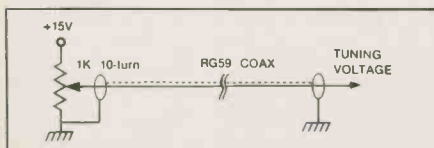
Fig. 4. The VCO tuning voltage wiring.
