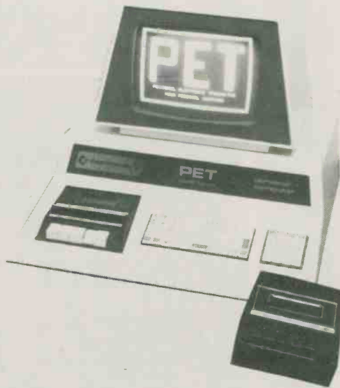
Cassette machines are a popular low-cost method of data storage. Their slow speed is a disadvantage.
