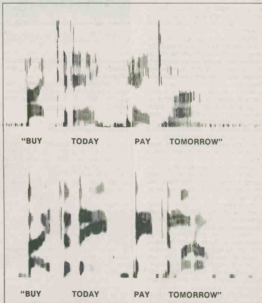
Voicegrams of two people speaking the same words with identical taping equipment show similarities as well as differences of pattern. The scientific question is how accurately prints can be identified or differentiated. In these samples time is measured horizontally for a duration of under 1.5 seconds, while frequency is scaled vertically with in a range of 4,000 Hz. Relative darkness indicates intensity.
