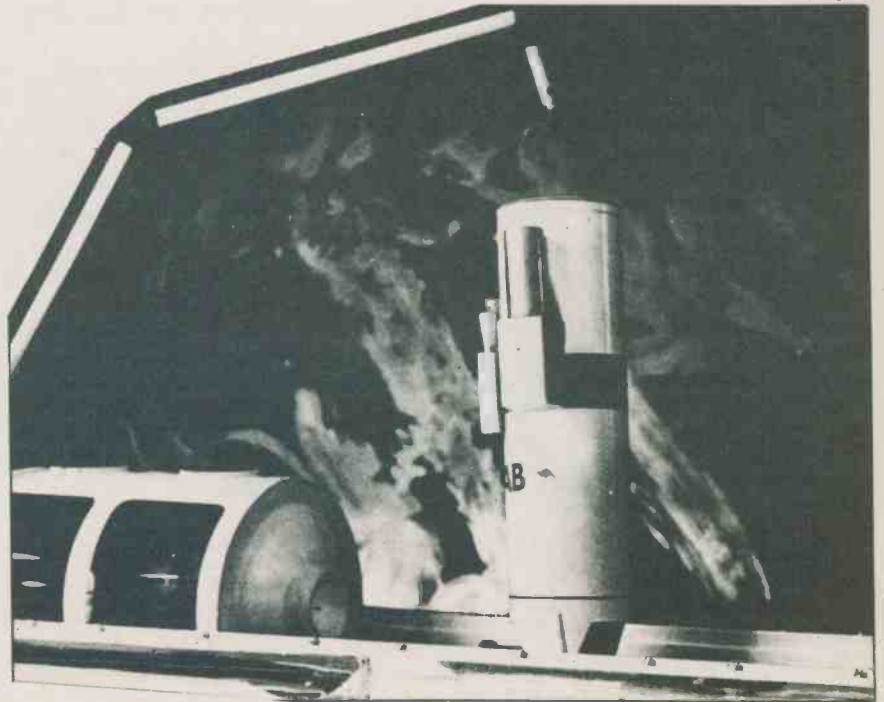
Mock-up model of Starlab being lifted out of the instrument bay of the Space Shuttle.
