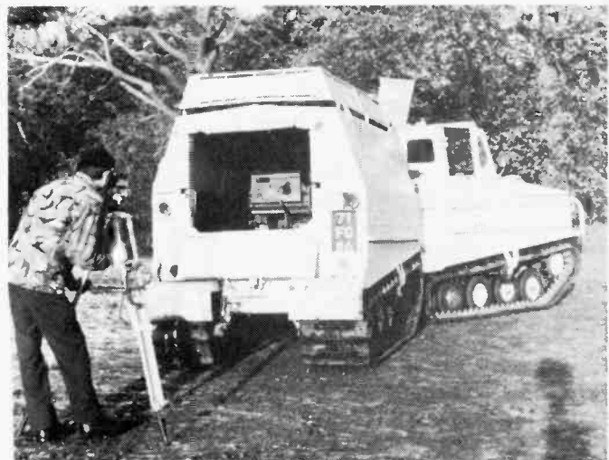
Ferranti PADS (Position and Azimuth Determining System). A digital inertial navigation system for accurate artillery survey purposes.
