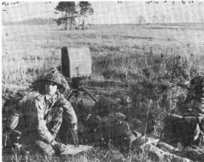
Above: The ZB298 is a mobile ground surveillance radar for the detection and location of moving targets.
