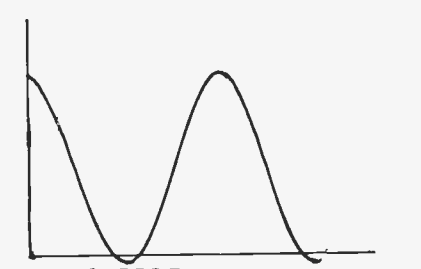
clamped at -0.6v by the bridge
