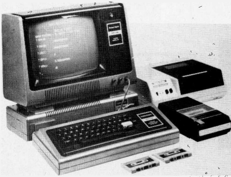
The TRS-80 CPU, the expansion interface (under the monitor), and the 'Quick Printer'. Plus cassette recorder and Radio Shack video monitor. Also in our Sample System is the mini disk system.
