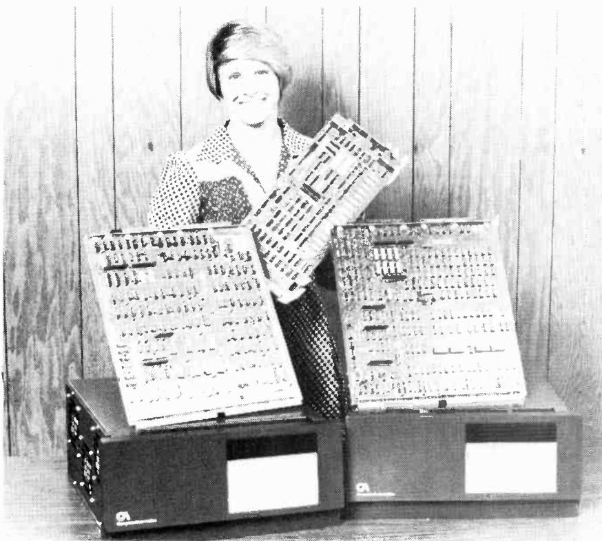
Naked Mini — 4 Family claimed to put an end to compromise in minicomputer selection by OEM and volume users through design modularity, upward and downward compatibility, exclusive input/output flexibility, and a very broad range of memory products. The Family computers are LSI 4/30, LSI 4/10, and LSI 4/90 (left to right). Packaged versions come in operator's (left) or programmer's console.
