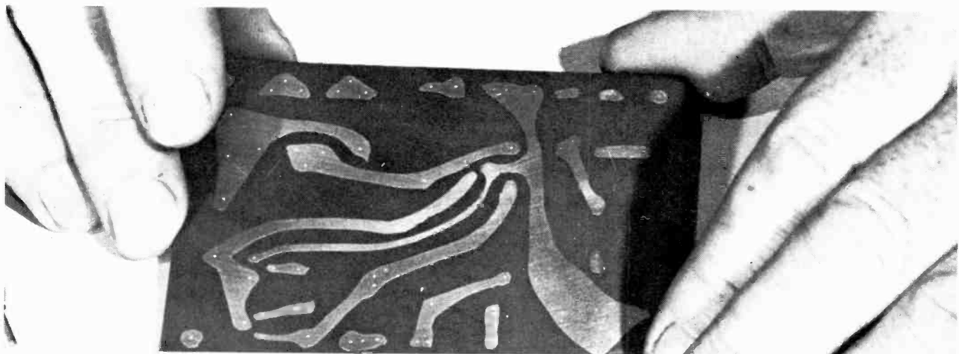
Fig. 11. The board, cleaned and ready for drilling.
