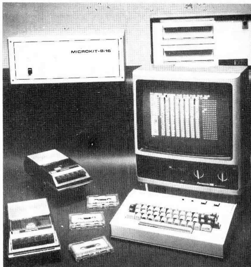
The Microkit 8/16 can incorporate either an 8080 or 6800 processor. Available software includes an excellent text editor.
