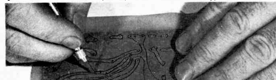
Fig. 7. Remove the unwanted film, leaving film over the areas where copper is to remain.
