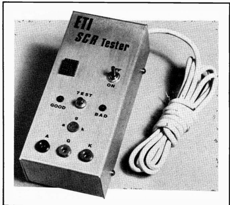
The completed unit is built into a strong aluminum box.
