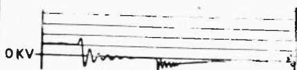
Unusual point opening signal (note hash extreme right of picture) burnt or arcing points.
