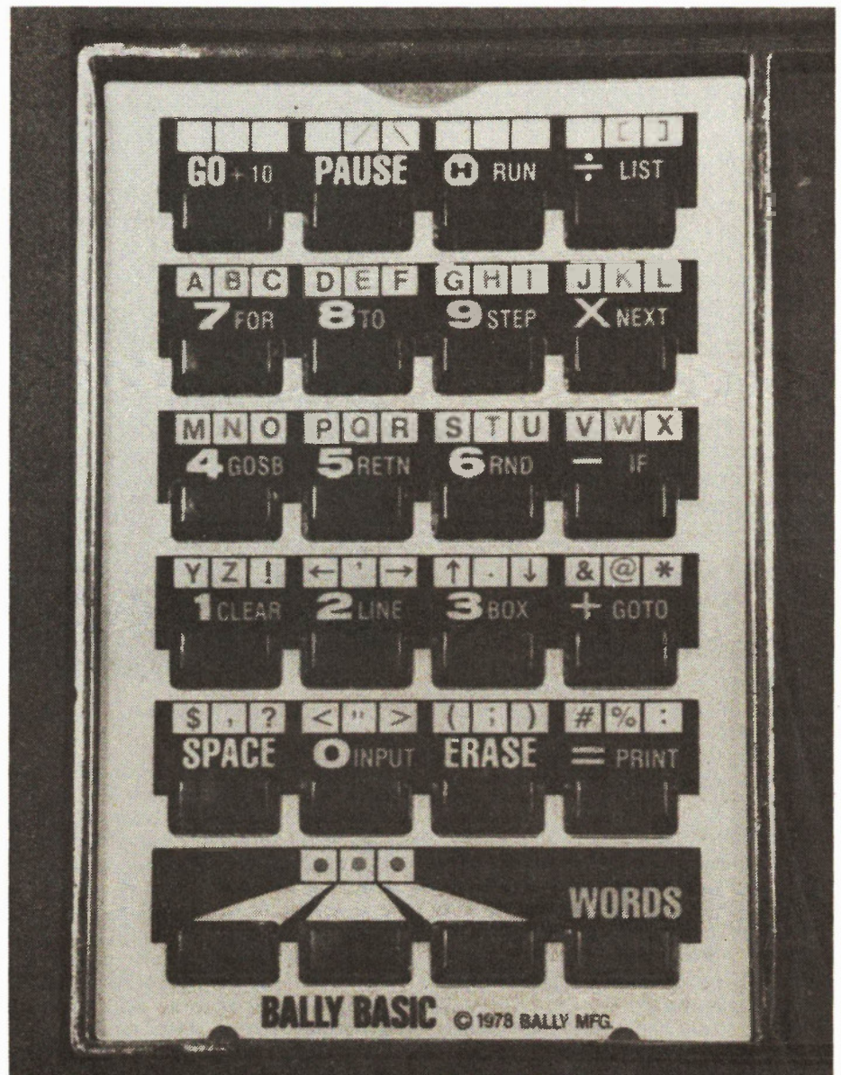
Fig. 5. BASIC overlay on keyboard shows functions and instructions available.
