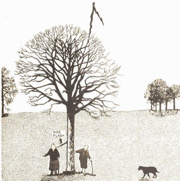
Side flash from a tree struck by lightning. At first the current flows through the trunk. The electrical resistance of the trunk, between ground and a point level with the head of anyone standing nearby, may be a few kilohms. Build-up of current through it may cause the potential drop across the lower part of the trunk to exceed the electrical break-down strength of the air between the trunk and the victim. At that stage a side flash occurs.
