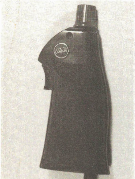
Fig. 2. One of two hand controls supplied with Arcade. Sockets on machine accommodate two more.
