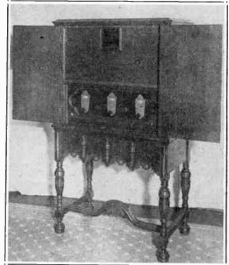
A combination radio eye for receiving Television and broadcast set. A snap switch changes the radio circuit from loud speaker to radio eye. The moving objects or animated picture appear in the opening of the timing control
