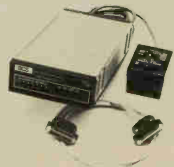
Billed as a first in the industry, Terminal Service Unit (TSU), designed by Boeing Computer Services for use with low-speed terminals uses local voice-grade telephone lines. Device provides error control, data quality monitoring and terminal usage statistics.
