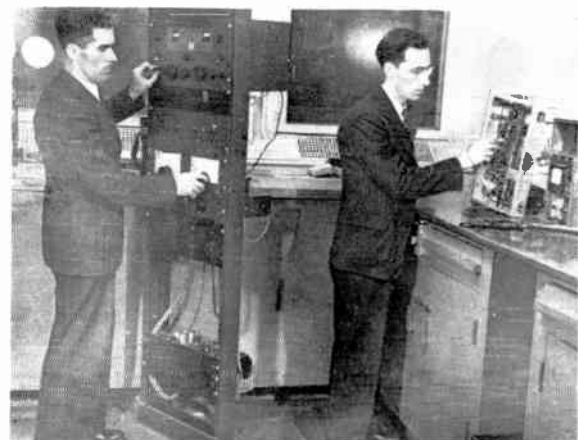
Sackville "lab" is completely shielded by two concentric layers of copper screening to isolate it from strong "fields" of transmitters and antennae to ensure accuracy of measurements and tests. Operations Supervisor Merrill Young measures frequency of transmitter on the frequency standard, while Operator Elmer Hughes checks performance of modulation monitor.
