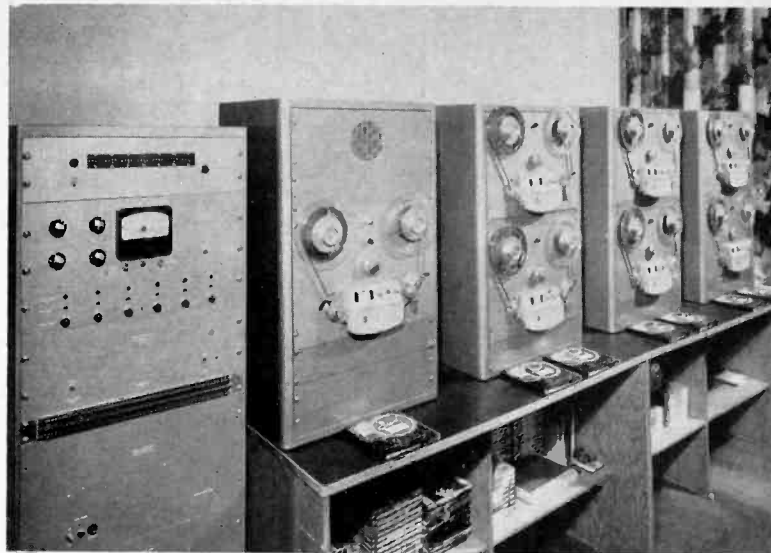
THE MULTIPLE TAPE duplicator seen here has produced more than 50,000 commercial hours of programs for Canadian stations. The equipment is capable of turning out three hours of programming every 15 minutes. It was custom tailored for S. W. Caldwell Ltd. by the Stencil Hoffman Corp. of Hollywood.
