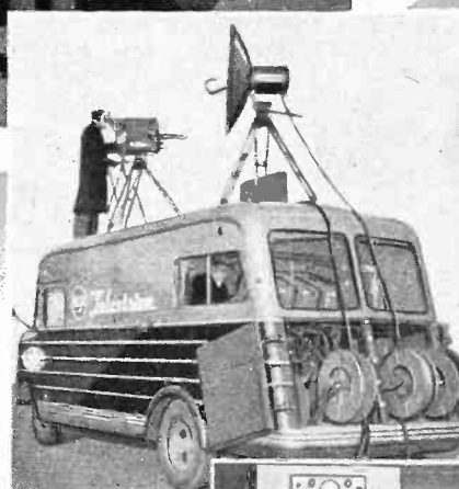
LEFT: The RCA Mobile TV-Unit ready for telecasting. The reinforced roof supports the cameras, relay equipment and operating personnel.
