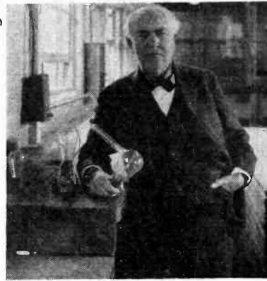
Photographed in 1912, with models of his "Edison Effect" lamps, is the forerunner of modern radio and other electronic tubes. The tubes were developed shortly after 1883, when Edison discovered that a heated filament in a vacuum tube emits electrons.
