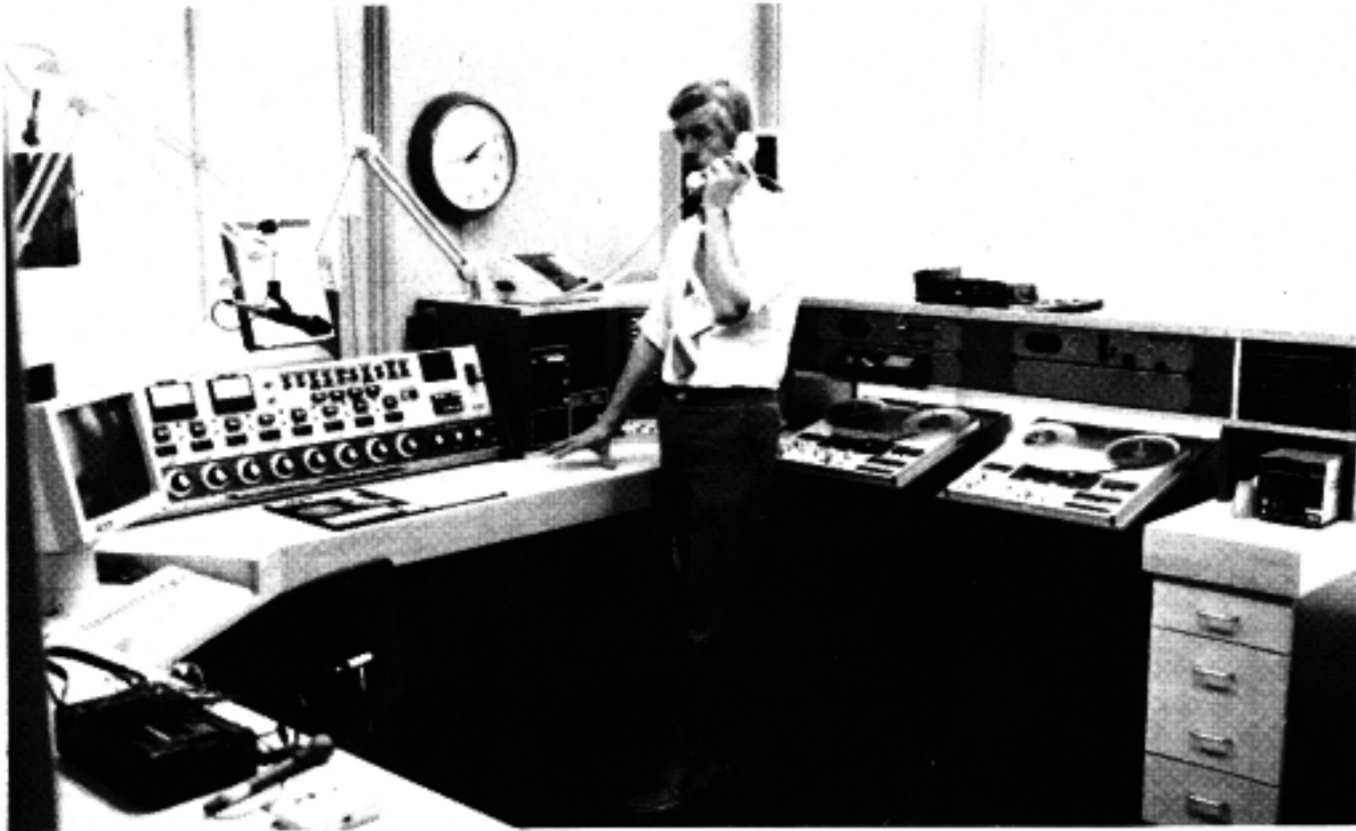
News studio. Using telephone is John Ashbridge, CKNW news coordinator. The console is a JVE 5050 built by John Visser Electronics. To the right are: the turret assembly which houses the ITC 3-deck recorder-producer unit; the modules containing the input selectors for the cartridge machine; the two Studer-Revox PR 99 tape machines; the Gentner SPH-4 telephone hybrid unit; and (above the tape machines) assorted monitor panels and scanners. To the left of the console is one of the Kimtron word processors.
