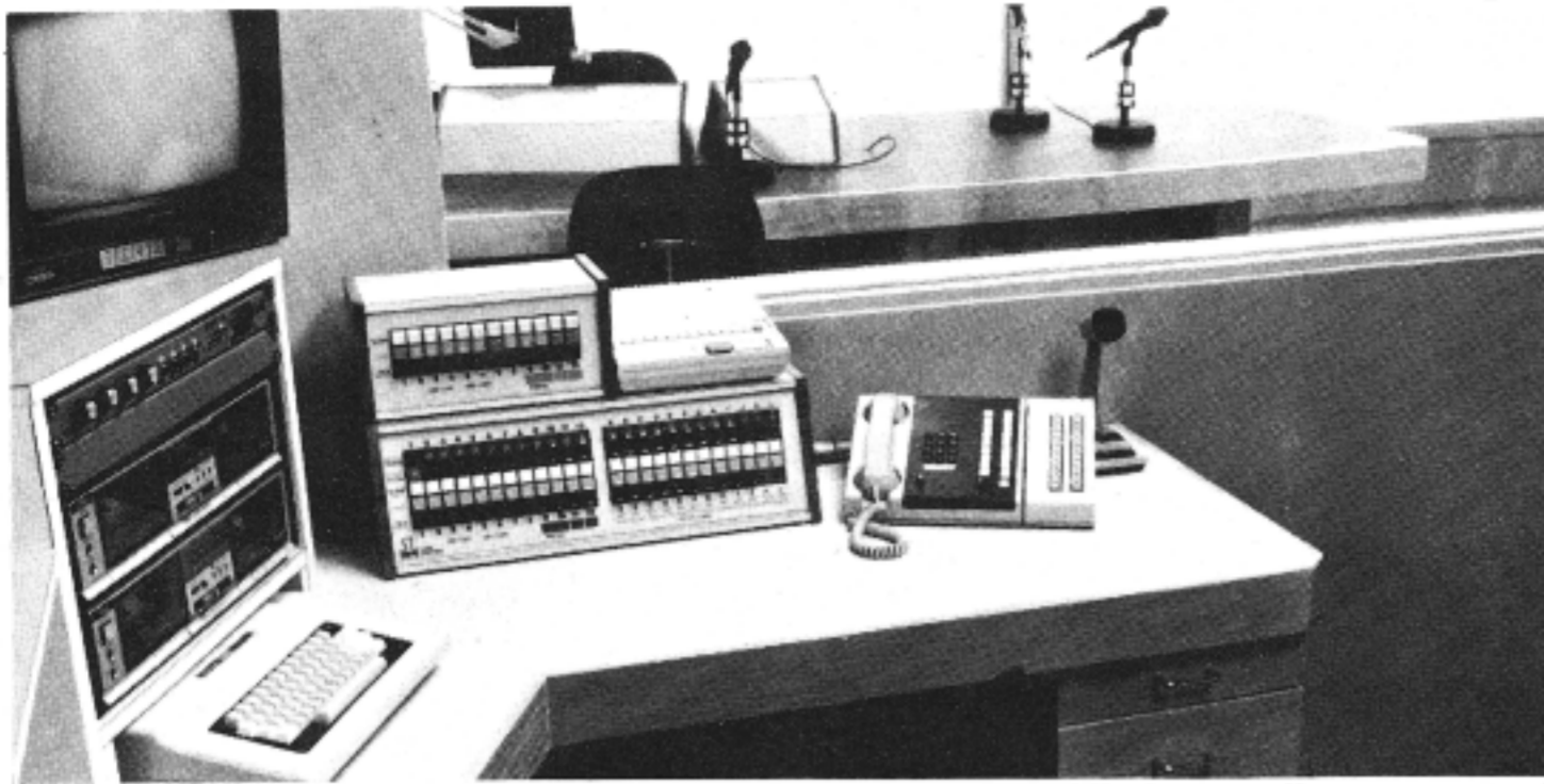
Screener-producer's position (looking into the main studio). All phone calls are screened by this producer, who makes the decision on whether the call is topic-related. If the call is suitable, it is transferred to the talk show host's position in the studio, where it can then be put on the air. The computer keyboard (left) is used for typing messages and information that will appear on the video monitor in the main studio. The screener also has the means to record and make tape cassette copies of programs in progress. The video monitor receives cable channels, which are then available to the talk show host on his video monitor. (Also available at this position is the intercom system to all exterior doors, along with electric latch door release buttons; a video camera input is provided for visual identification of guests at the exterior doors.)
