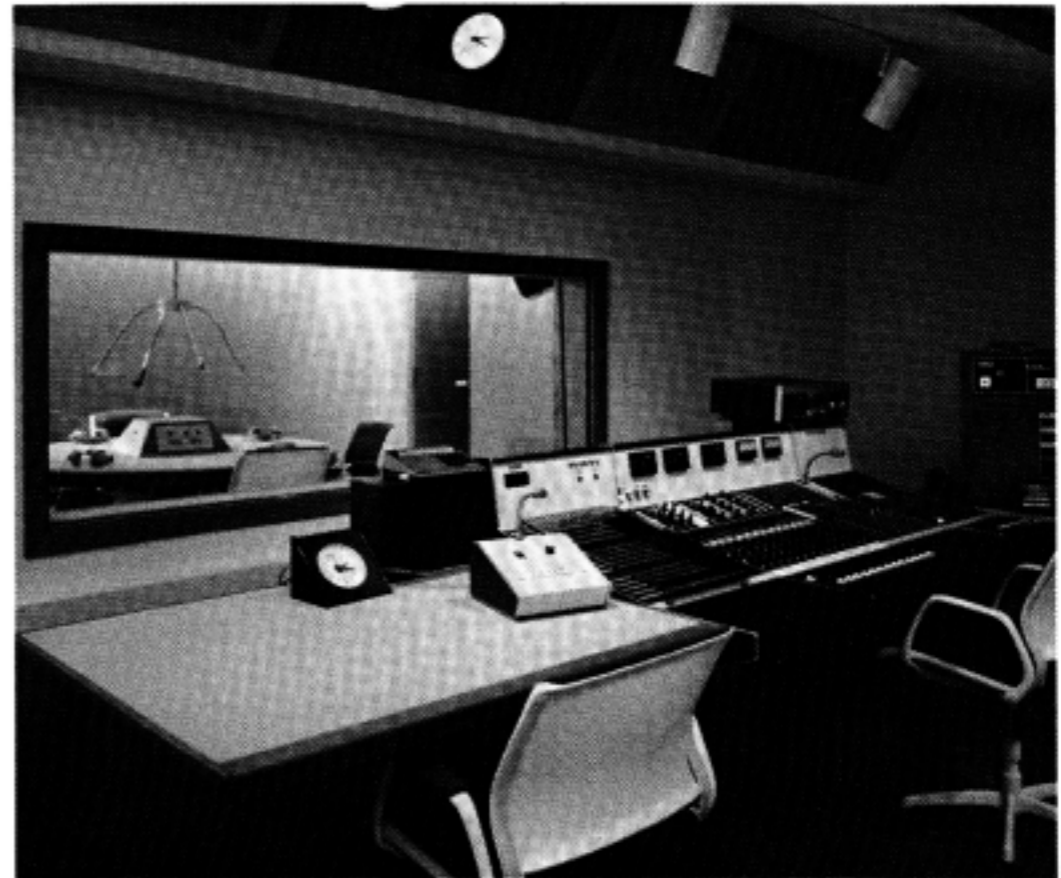
Control rooms have been designed for an ambient noise level of NC-25 and reverberation time of 0.35 secs. Walls are non-parallel, with reflective sloped butterfly ceiling. Equipment includes Ward-Beck 14-input consoles (expandable to 20), two turntables, 3 tape recorders, 2 cartridges, 1 cassette unit, Canadian-made PSB passif I speakers and special integrated intercom. Note suspended condenser mic set-up, with turret for controls.
