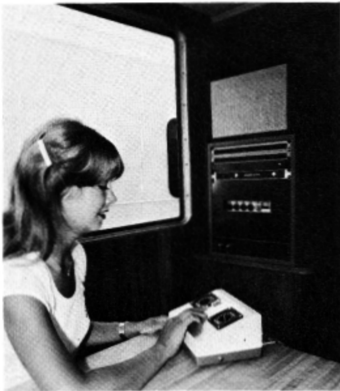
Photo shows interior of mobile unit constructed by Ontario Motor Homes for CHIN Radio in Toronto. The Itasca 26RG Winnebago unit has been remodelled to provide reception area and soundproof studio having large double-glazed windows on three sides, lead sheeting on fourth. Generator compartment is also lined with lead to isolate noise. CHIN engineer Trevor Joyce says self-driven vehicle replaces trailered unit, providing greater mobility for on-location broadcasting.
