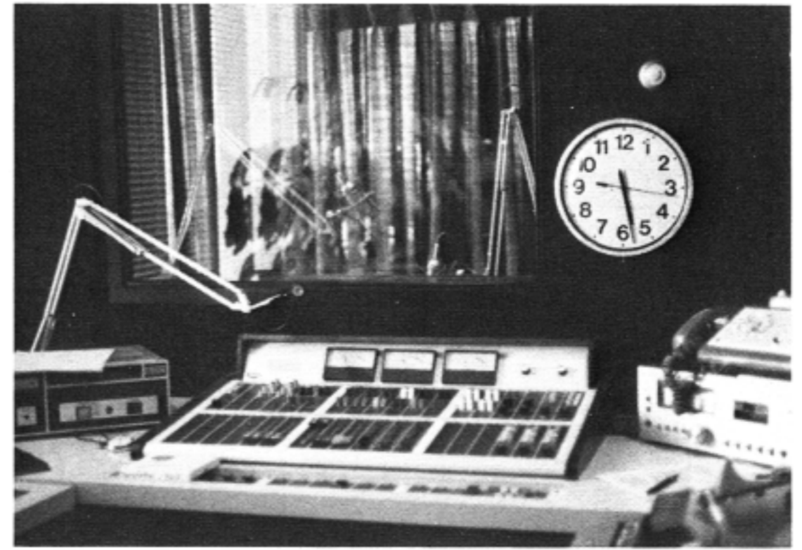
On-air control room (left) and production control room (right) at Q-107 are equipped with McCurdy SS-7600 stereo consoles, Technics turntables.
