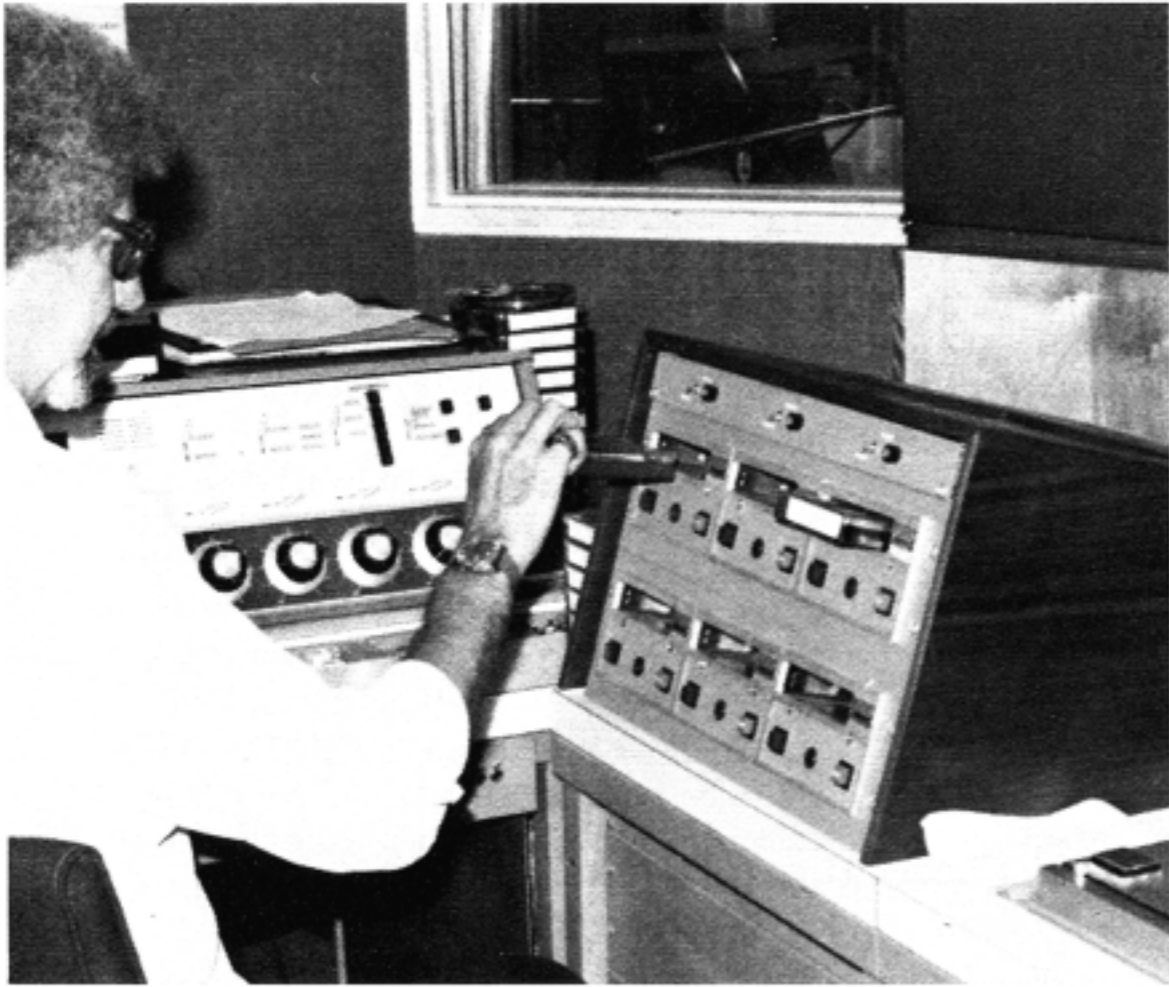
Phase shift which degrades conventional duplicating has been eliminated in a system using UMC Beaucart type 10 reproducers, developed by Ron Turnpenny vice president of engineering at CHFI-FM, Toronto.
