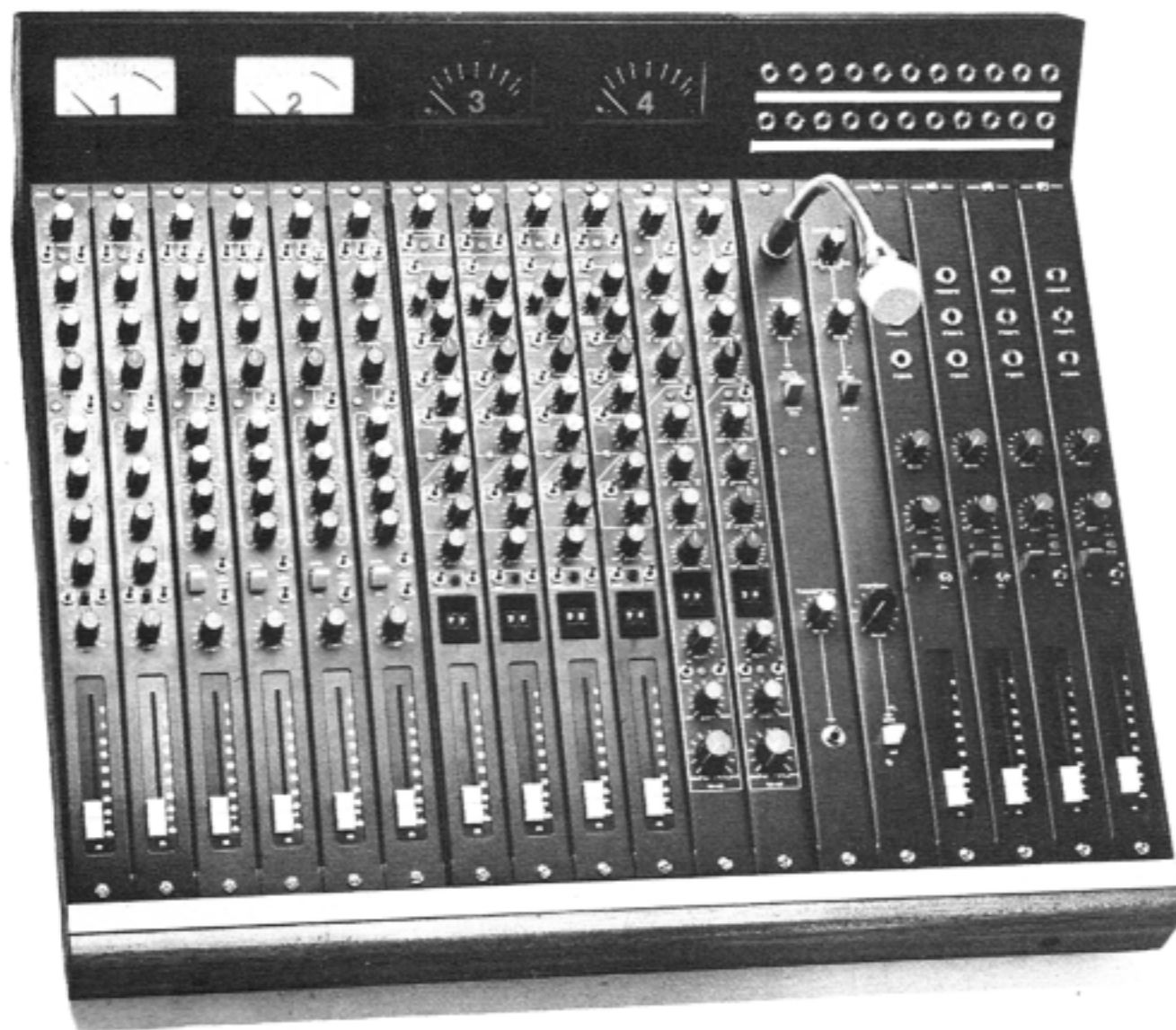
SHOWN ABOVE: Midas 3 bay console containing the following complement; 2 x PRO 02,4 x PRO 03,4 x PRO 04 Input Modules; 2 x PRO 09B Echo/Foldback Master Modules; 1 x PRO 20 PFL/Talkback Module; 1 x PRO 21 Monitor/Oscillator Module and 4 x PRO 11 Submaster/Output Modules. Shown fitted with simple patch bay, VU and PPM metering.
