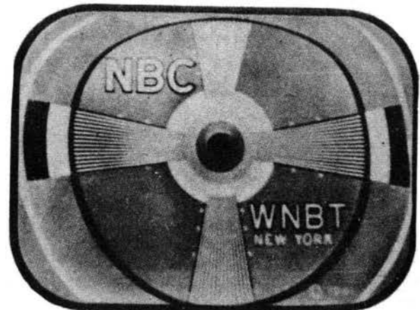
Fig. 20 Vertical Linearity Control Misadjusted
