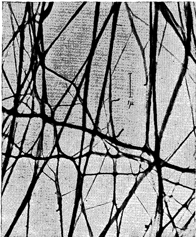
FIG. 20.39a.—Soap-curd fibers. Picture taken with the electron microscope. Magnification is about 10,000 times: 1\mu = 1 micron = 10^{-6} meters. (Courtesy of J. W. McBain.)
