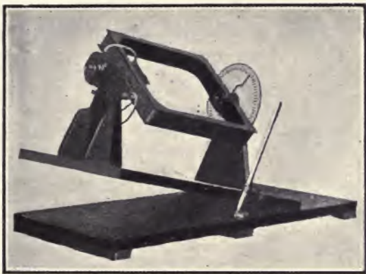
FIG. 49.—Photograph showing details of construction of the Tilting Receiving Coil, L_2 .
