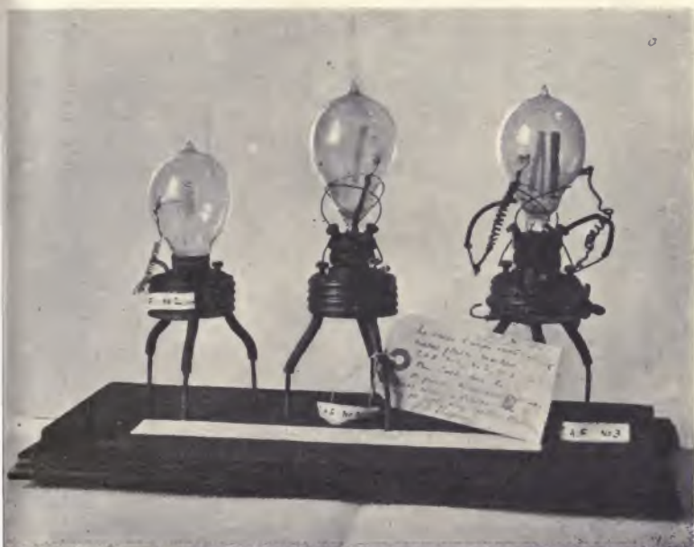
FIG. 28.—Photographs of the original Valves used by the Author for rectifying electric oscillations in 1904.
