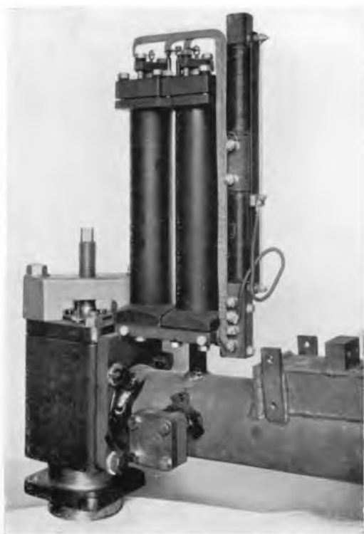
FIG. 68.— A typical Pirani vacuum gauge and main vacuum valve. (B. T-H.)
