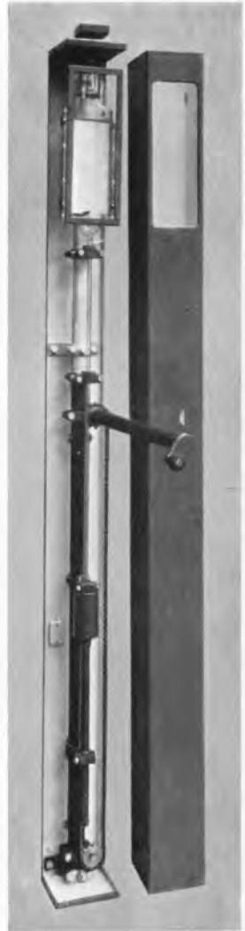
FIG. 66. — A typical McLeod vacuum gauge with the cover removed.
