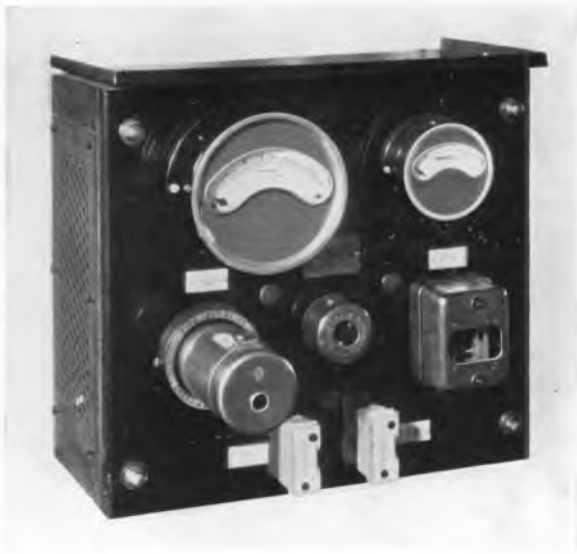
FIG. 68A. Typical Pirani vacuum gauge instrument panel. (B. T-H.)
