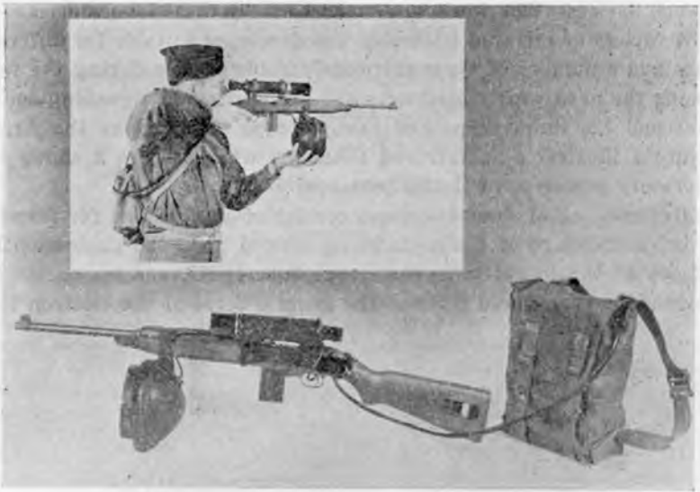
Fig. 2—Laboratory prototype sniperscope.
