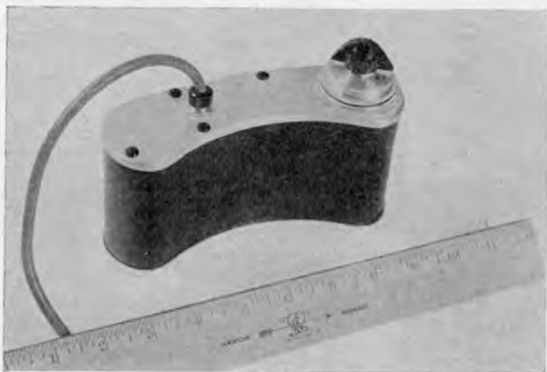
Fig. 15—5-kilovolt vibrator power supply.
