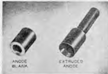
Fig. 9—Fabrication of anode.
