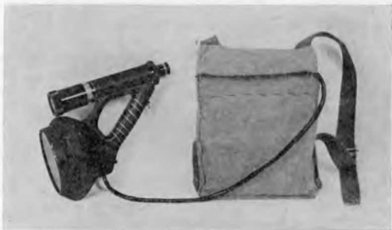
Fig. 9—Laboratory prototype Snooperscope.
