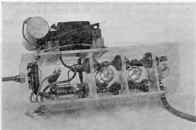
Fig. 23—16-kilovolt voltage quadrupler power supply.
