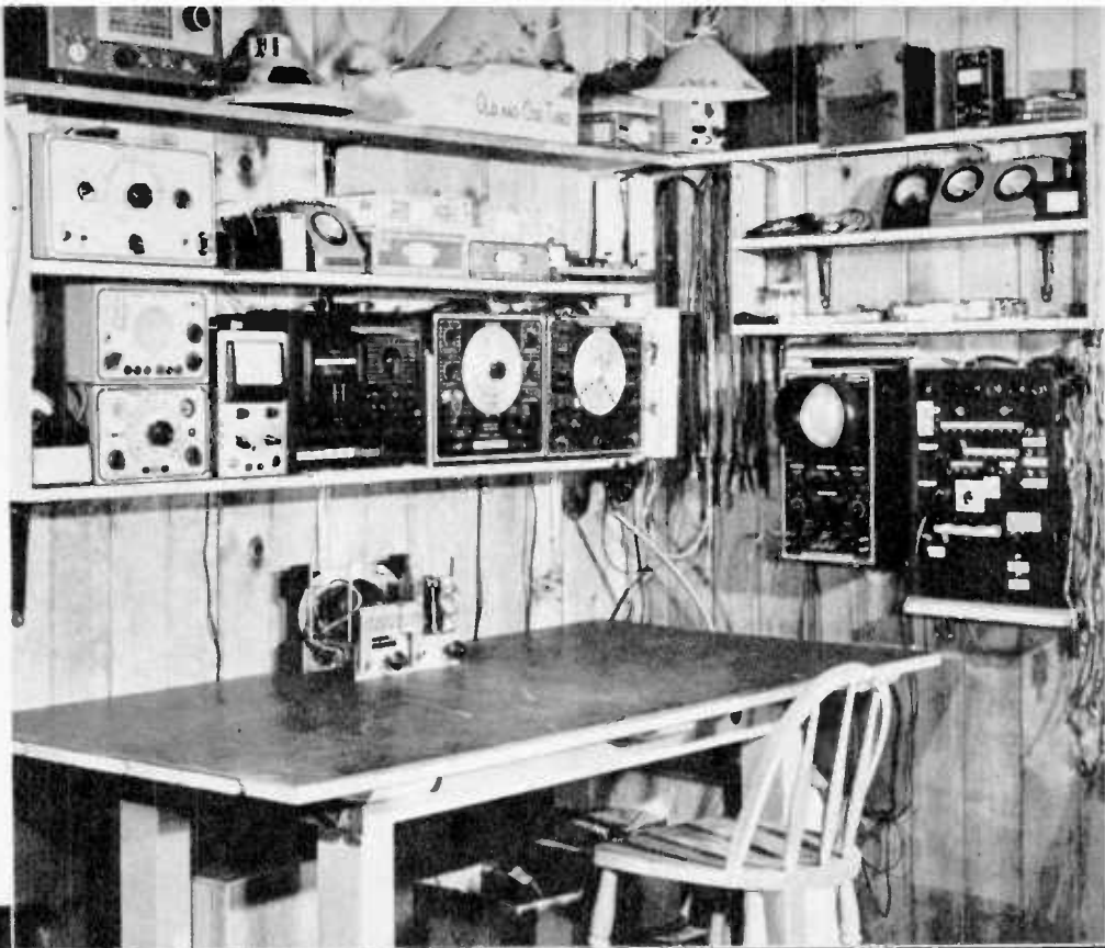
ON CASTERED TABLE (photo left) this 5-inch scope is easily, quickly moved to convenient position next to workbench. Bottom shelf holds speaker. Although 19 inches deep, cathode-ray oscilloscope (second from right, above chair in photo above) occupies little wall space. Body of scope is behind wall. Opening in wall is one inch larger all around body, so scope can be removed easily for inspection, cleaning. Lead-in wire of radio or TV aerial (photo below) can conduct rain as well as entertainment into house if run straight through window. Always form loop in it, to allow water to drop off harmlessly.
