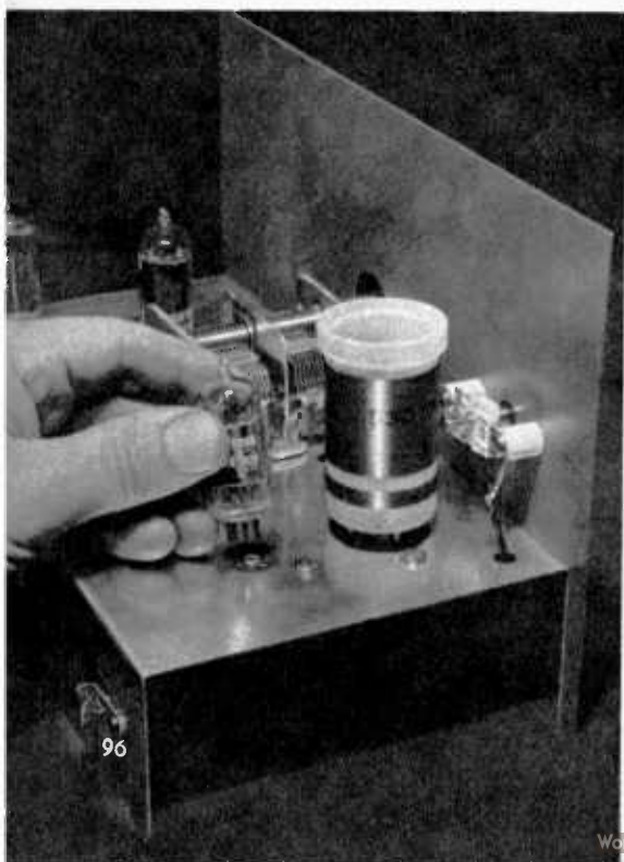
PLUG-IN COIL , held in hand at right (photo above), fits into five-prong socket on chassis. Loud-speaker connects to two screw terminals on back edge, earphones to tip jacks to left, and aerial to spring binding post on right. The combined detector-first amplifier tube, a 12AT6 (photo below), goes into socket directly behind plug-in coil. Unit to right of coil is antenna trimmer capacitor, which is adjusted from front.
