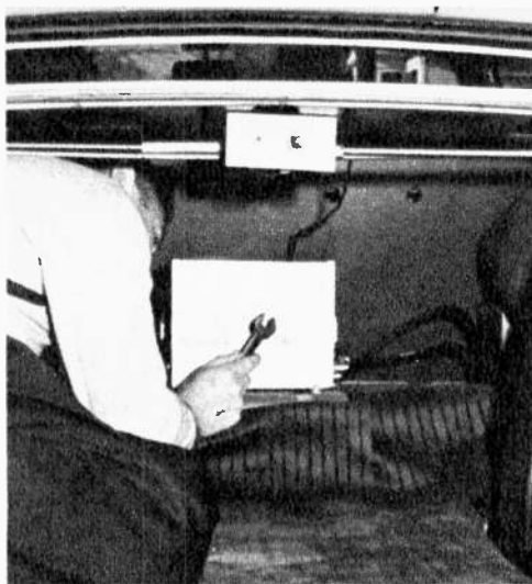
PART OF TRANSMITTER (the power supply and modulator section) is mounted in trunk compartment. It is operated automatically when the push-to-talk button on hand microphone is pressed.
