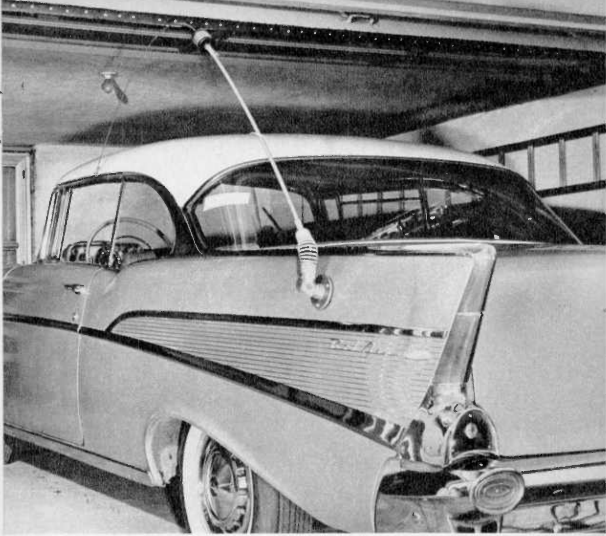
GETTING IN AND OUT of the garage is no problem with tip of antenna clamped to rain molding of car.
