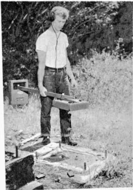
THE FISHER MODEL ME locator (photo above) discloses the presence of an overgrown tower base through its large iron bolts. It's easy to handle.
