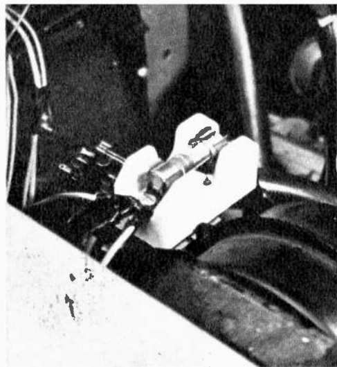
SHORT-WAVE EQUIPMENT is connected directly to battery (through ammeter) and through these protective fuses, mounted on blower frame under hood. These extra fuses protect the ignition system.
