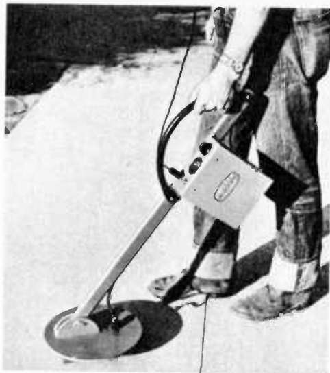
HIDDEN "TREASURE" is often something like a water or gas pipe, which must be located for replacement, etc. Used here: Fisher Model T-10.
