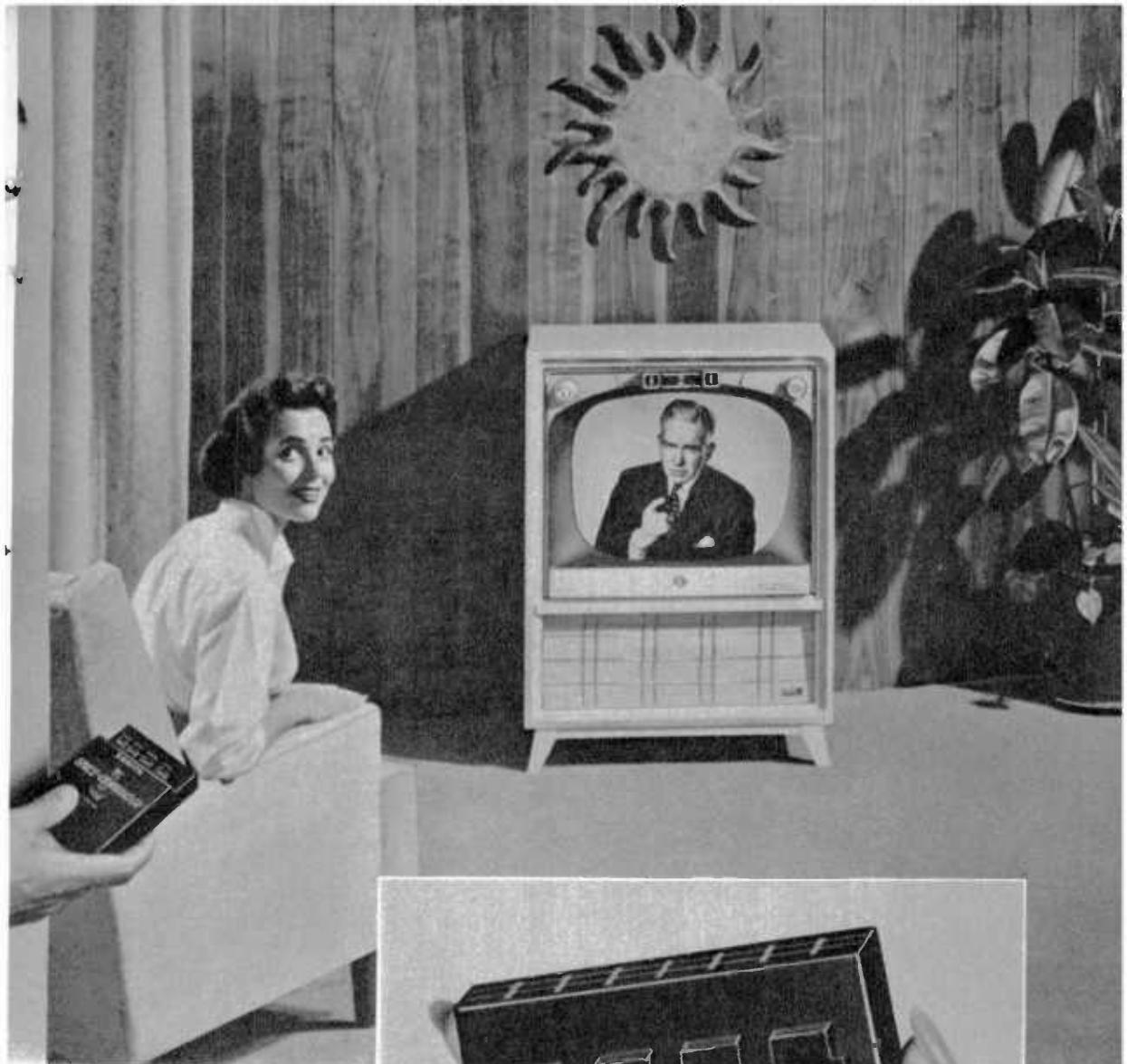
"SPACE COMMANDER" unit is simplicity itself. Ultrasonic impulses come out of the open grille area at top of the case. Page 26 shows the operation.
