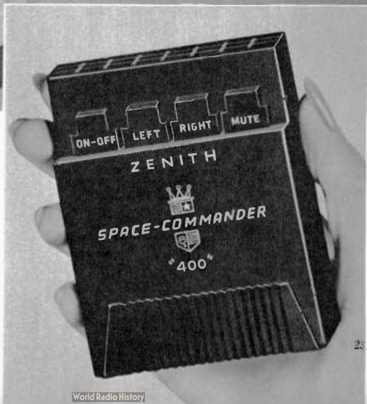
"SPACE COMMANDER" unit is simplicity itself. Ultrasonic impulses come out of the open grille area at top of the case. Page 26 shows the operation.
