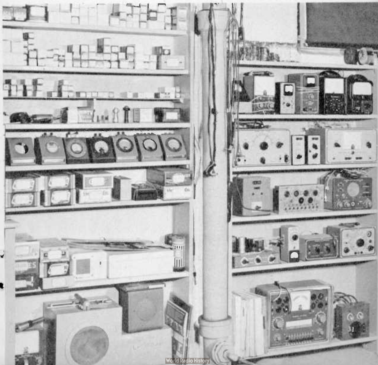
THESE racks contain miscellaneous meters and test equipment, spare parts and replacement tubes. Most equipment was assembled from kits. Shallow shelf arrangement makes all units readily accessible. Equipment shown represents accumulation of about 10 years. Is more elaborate than needed for service work.
