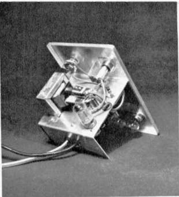
CONELRAD chassis, top view, completely wired. Thyatron tube is in the right front corner. Bottom wires are for AC power and AVC voltage from set.
