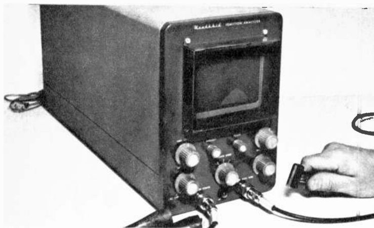
THE HEAVY TEST leads of the analyzer are 10 feet long, permitting the instrument to be set up on a bench adjacent to the car. The low-voltage breaker point lead, with its two connector clips, is on the left. On the right, the hand is holding the paper clip that goes around but does not connect to a spark plug wire. Front panel controls of ignition analyzer are similar to those found on standard oscilloscope.
