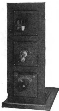
Fig. 30.—Unit Type Construction is Employed for This Receiving Set.
