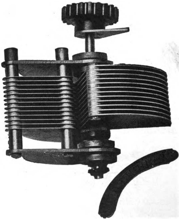
Fig. 29.—A Close-Up View of the De Forest Army Type Variable Condenser.
