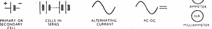
PRIMARY OR SECONDARY CELL CELLS IN SERIES ALTERNATING CURRENT AC-DC AMMETER MILLIAMMETER
