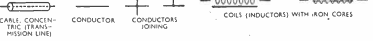
CABLE, CONCENTRIC (TRANSMISSION LINE) CONDUCTOR CONDUCTORS JOINING COILS (INDUCTORS) WITH IRON CORES
