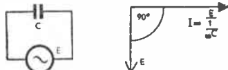
Fig. 32. (Left) Alternating voltage applied to capacitance. Fig. 33. (Right) Voltage vector lagging current by 90^\circ .
