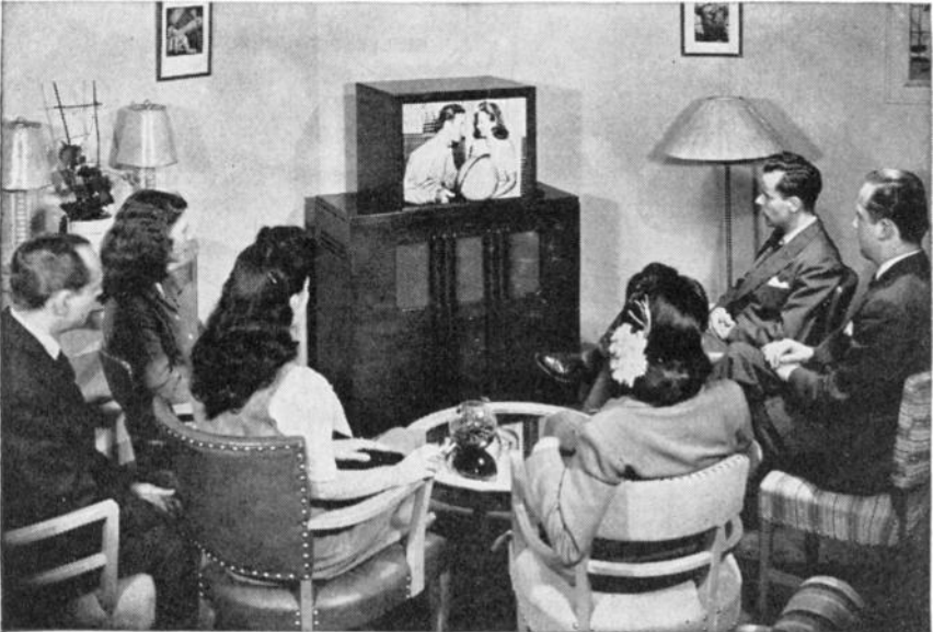
Fig. 8.42B. A large screen (20 by 16 inches) receiver. The image from a small projection-type tube is enlarged to permit comfortable viewing by many people.
