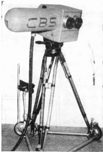
FIG. 15.2. A color live pick-up camera using an Orthicon tube.
