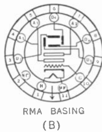
FIG. 8.7. The basic elements of a cathode-ray tube (A). The great number of elements found in these tubes necessitate a larger tube base, as shown in (B).
