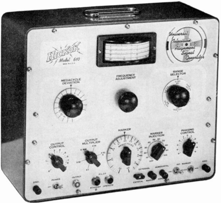
FIG. 11.15. A signal generator covering the F-M and television bands.
