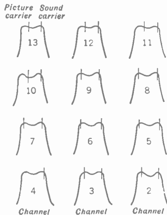
Fig. 11.23. The R.F. response characteristics of the RCA receiver.
