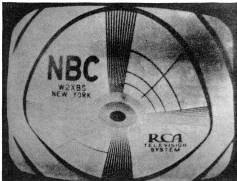
FIG. 14.5. Unfiltered A.C. ripple in vertical deflection amplifiers.
