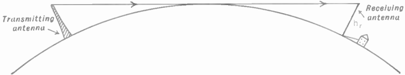
FIG. 2.6. Increasing the line-of-sight distance from the receiving antenna to the transmitter by raising both structures as high as possible.
