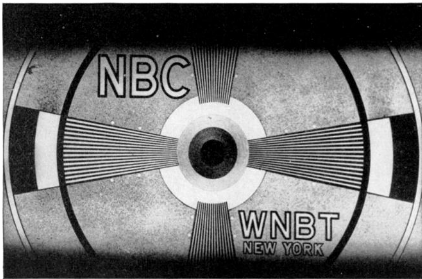
FIG. 14.6. A large percentage of ripple voltage in the video amplifiers.
