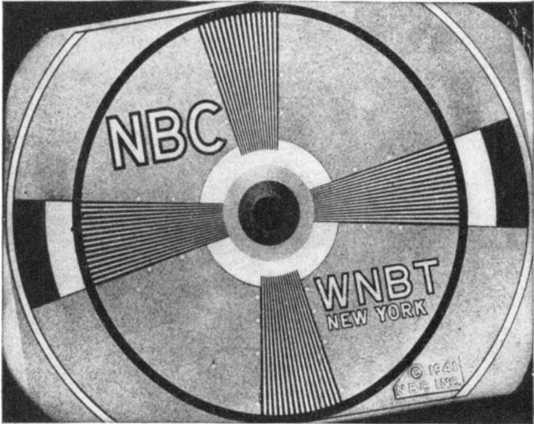
FIG. 8.16. Incorrectly positioned image due to improper placement of deflecting coil yoke.
