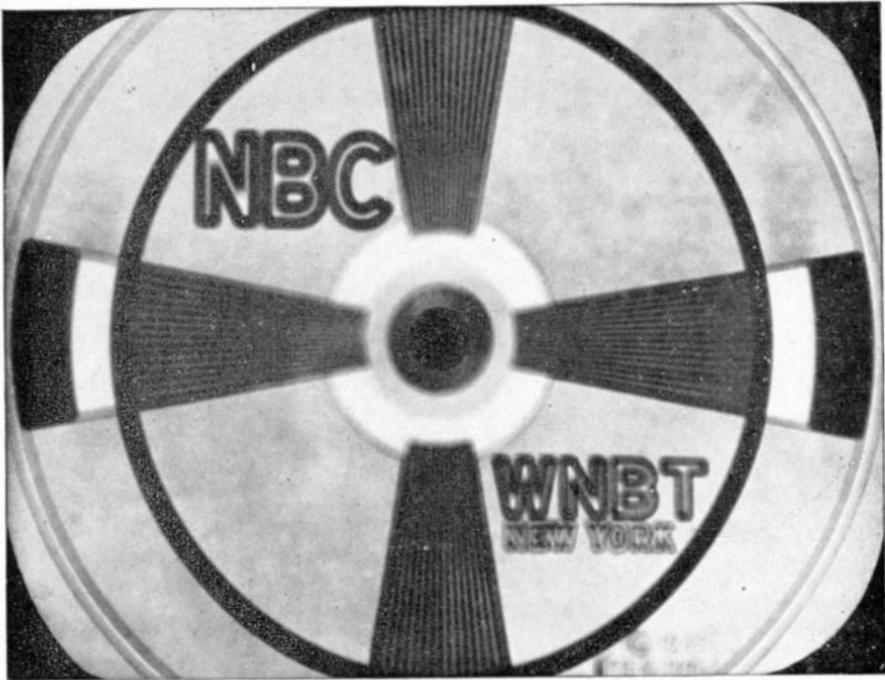
FIG. 14.20. Distortion due to poor high-frequency response of video amplifiers.
