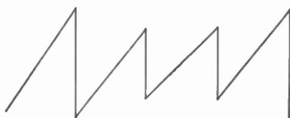
FIG. 14.17. A type of saw-tooth voltage variation that would cause patterns similar to that of Fig. 14.16.
