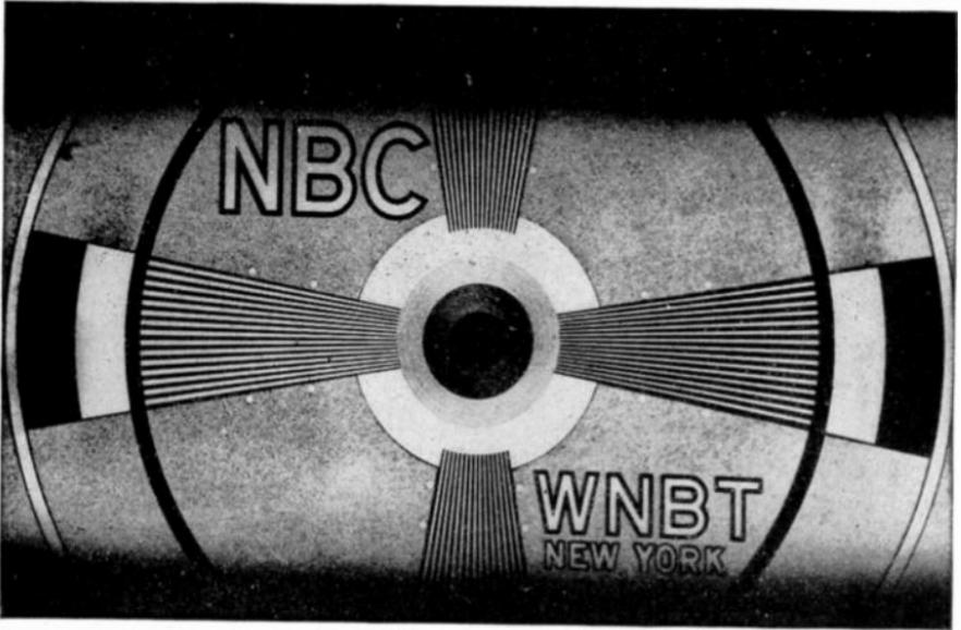
FIG. 14.4. A large percentage of ripple voltage in the video amplifiers.
