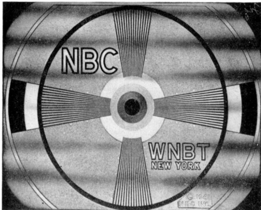
FIG. 14.5: The visual result when sound voltages reach the cathode-ray tube.
