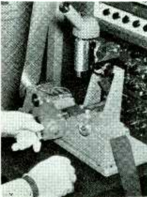
(I) Insert splicing tape beneath the lifted ends of the two tapes to be joined.
