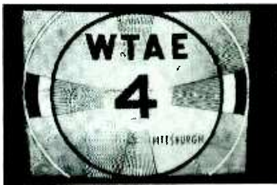
Fig. 11-30. Monitor display of poor signal-to-noise ratio caused by slight mistracking.
