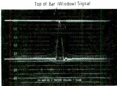
Fig. 12-7. Waveform-monitor display during playback of 2T-pulse, high-band standard.
