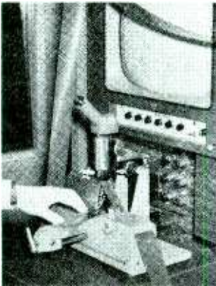
(E) Drape tape from supply reel over tape support post and position under left hold-down door.
