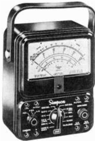
Fig. 11-4. The Simpson 260, a 20K ohms-per-volt multimeter. (Simpson Electric Company)
