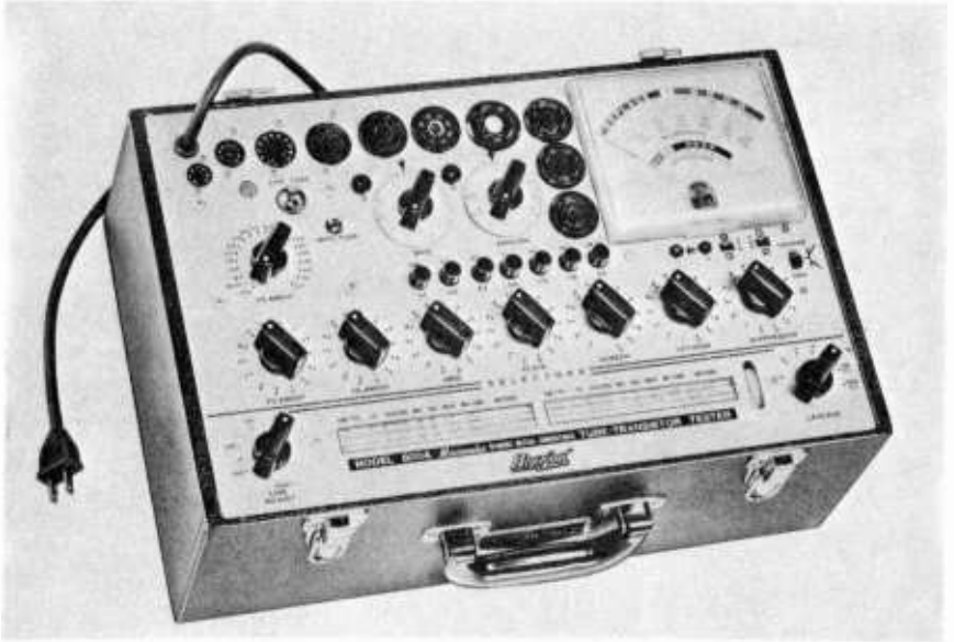
Fig. 11-6. The Hickok Model 800A dynamic mutual conductance tube-transistor checker. (Hickok Electrical Instrument Co.)
