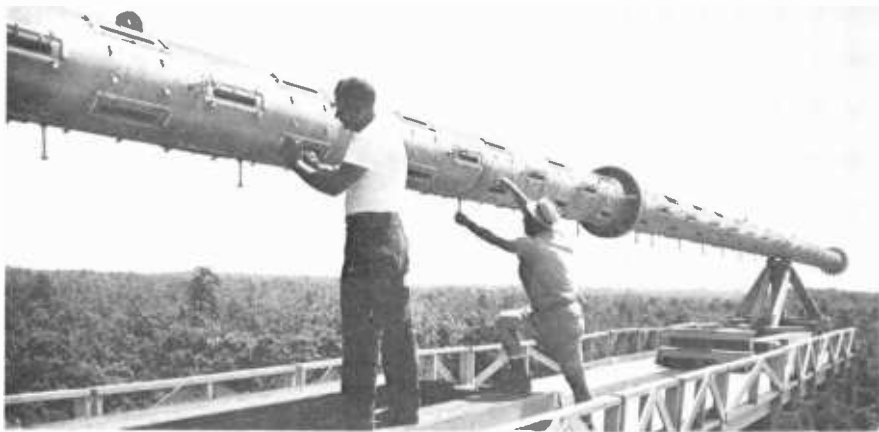
Fig. 7-13. This high-gain uhf pylon antenna is being readied for check-out on the turntable at the factory. The window covers are not yet in place. (RCA)
