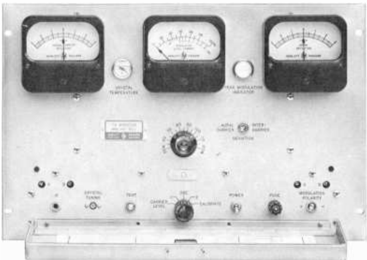
Fig. 5-12. The Hewlett-Packard 335E TV station monitor. (Hewlett-Packard)
