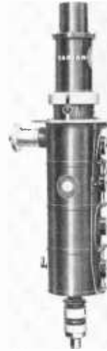
Fig. 5-7. The Varian klystron tube, used in high power RCA uhf transmitters, has four internal cavities. (RCA)
