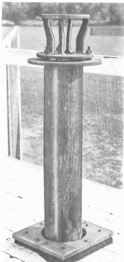
Fig. 4-27. The camera mount on WLBC-TV's camera platform. Note the rubber shockmounting where the pole comes through the platform floor. (WLBC-TV, Muncie, Indiana)
