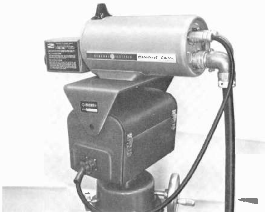
Fig. 4-3. A transistORIZED studio vidicon camera designed for remote control use, the GE PE-22A. Note that there is no viewfinder. (GE)
