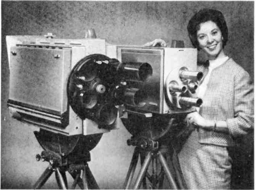
Fig. 3-12. (left) General Electric's model PE-20 image orthicon camera. (right) General Electric's model PE-23 studio vidicon camera. (GE)
