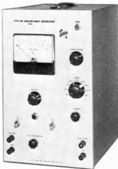
Fig. 11-9. The Tektronix Square-Wave Generator, Type 105. (Tektronix, Inc.)
