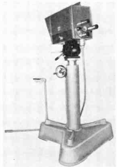
Fig. 3-14. This Sarkes-Tarzian studio vidicon camera uses a 1-inch vidicon tube. (Sarkes-Tarzian, Inc.)
