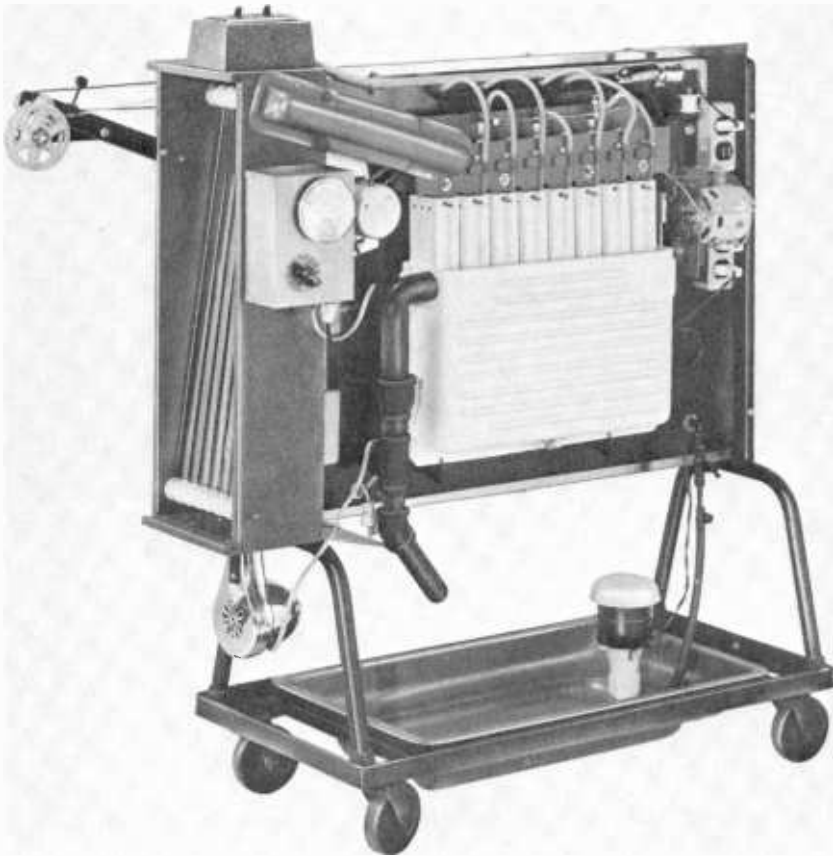
Fig. 8-16. The Cramer 60-1, a 16 mm film processor for both negative and reversal film. (Milco Manufacturing Co.)
