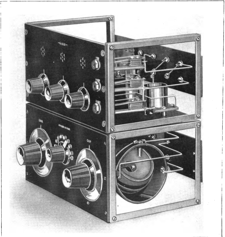
Fig. 1. A 150- to 2,600-meter receiving set which can be assembled with no other tools but a hand drill, screw driver, pliers, and soldering iron.
